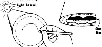
Run a bead of Superbond along the body and inside the cylinder joint as shown above. Smooth the glue with your finger. When thoroughly dry the assembly will be rigid enough so that the final trimming away of the membrane can be performed.
