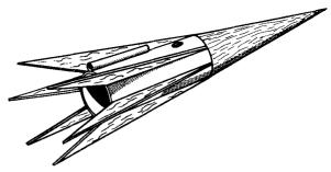
When entirely dry the cockpit assembly should be sprayed (or brushed) with your favorite color. Our favorite paint pattern is all white with a red point on the top  $1\frac{1}{4}$  of the nose. This does not have to be carefully masked as the self-sticking cockpit pattern assures a clean line. Note that the empty engine casing serves quite well as a support for holding the assembly during painting.
