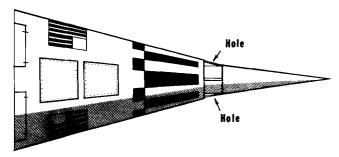
The nose cone now can be gripped for easier final alignment. This is done to insure that the engine thrust will not be cocked off to one side during flight.
