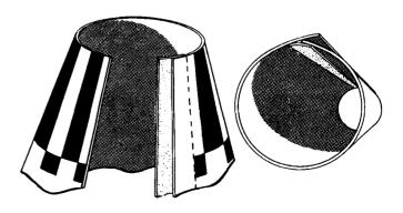
The tape is used to key the joint in place prior to any gluing. First tack the small end of the cone together, then key in the large end, and finally connect the entire seam in its proper place.
