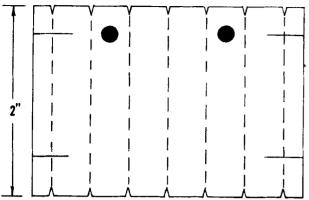
At this time, also use the guide to mark the  $2\frac{1}{4}$ " long body tube for cutting down to a 2" length.
