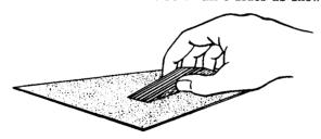
While still holding the 6 supports together, apply a thin film of glue to the edges which will be bonded to the tube.
