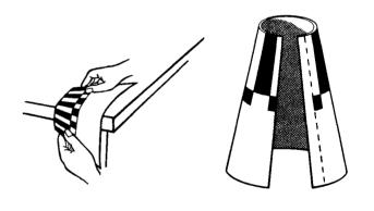
Apply Scotch tape the length of the entire seam as shown.
