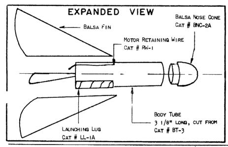
AS YOU WILL NOTICE, THE FINS ARE DESIGNED IN SUCH A WAY AS TO PROVIDE A HOLDER FOR A BOOSTER STAGE. FOR BOOSTER DESIGN. SEE OPPOSITE PAGE.
