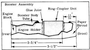
Wrap a layer of cellophane tape tightly around the joint of two rocket engines and slide them into the lower stage. Using your little finger or a brush, smear glue around the inside of the 6-1/2" long upper stage body tube to cover an area approximately 2" from one end of the body tube. Insert an engine block into the body tube and push it into place with the taped engines
