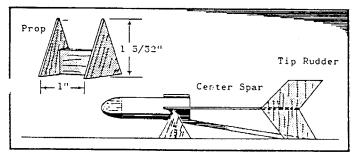
Cut two triangle shaped pieces of wood from scrap measuring  $1\ 5/32$ " from base to top. Glue these pieces to a l" piece of scrap to form a prop to align and support the engine tube assembly at the center wing roots while the rudders are being glued into position on the center wing tips. The bottom edges of the rudders must rest squarely on the table top as is shown. Let this assembly dry thoroughly before moving.
