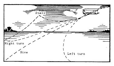
For example: Your model drops quickly and to the right. Cut a sliver of lead from the NCW-1 (only experience can tell you how much) and attach it near the trailing edge of the lower wing perhaps an inch left of the center.
