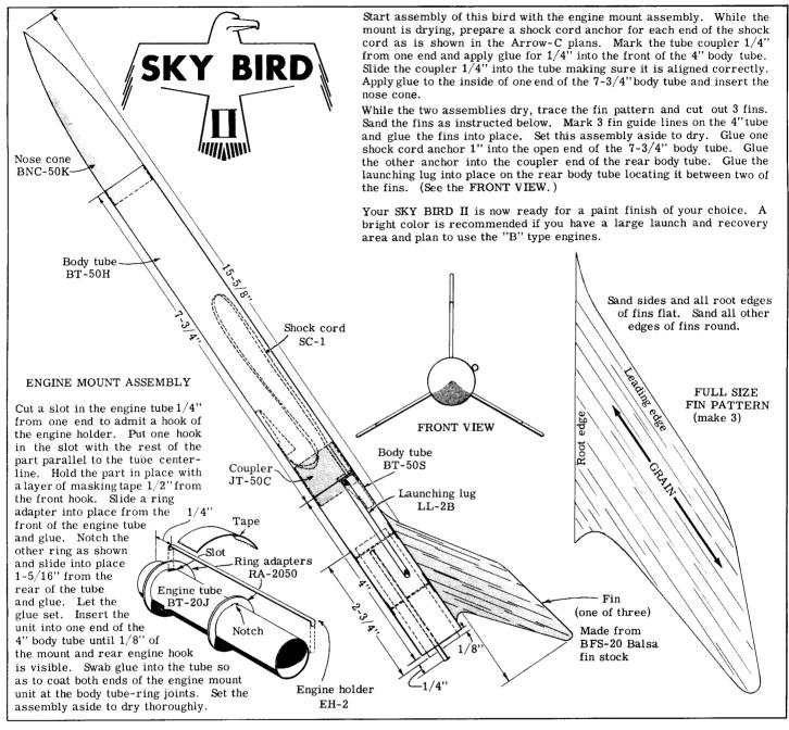
To obtain a good glue joint, the fin root should be sanded square and covered completely with glue before it is pressed in place against the body tube. After this glue has dried, a glue filler (fillet) is applied to the joint as shown. The rocket should be supported on its side while the glue dries.
