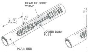
A. Make a mark 2 1/2" (6.4 cm) from the plain end of the Lower Body Tube along the seam of the body wrap.
