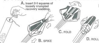
E. Wrap lines loosely around 'chute. Insert 'chute, shock cord and nose section into body tube.
