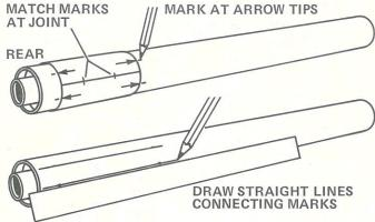
10 Cut out the body tube marking guide from the pattern sheet. Wrap it around the rear of the main body. Mark the tube at each arrow point, front and rear. Draw a straight line connecting each matching front and rear mark. (Use a ruler when drawing lines.) Extend the launch lug line forward 7". Mark the booster tube for four fins in the same way.
