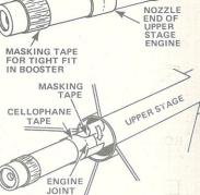
T-11 Slide the booster into place on the engine unit from the bottom. Position it so the stage coupler fits all the way into the upper stage and the fins are in line. Secure the booster in place by wrapping a layer of masking tape around the end of the engine mount tube and the engine. Press the tape down tightly.
