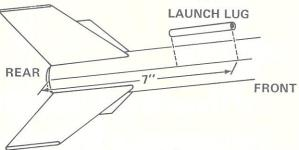
13 Glue the launch lug (part K) to the main body on its line. The front of the lug should be 7" from the rear of the body. Align it straight on the body.
