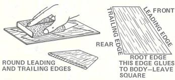
11 Fine sand the balsa sheets (part J), then carefully remove the die-cut fins from the sheet. Free the edges with a sharp knife. Sand the leading and trailing edges of the fins round. Leave the other edges square.
