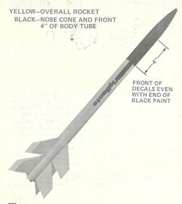
16 When all glue on the outside of the body is dry, prepare the model for painting. Apply at least two coats of sanding sealer to all wood parts. Let dry and sand lightly between coats. Do this until the tiny holes in the wood are filled and everything looks and feels smooth. Paint the entire rocket yellow. When the yellow is completely dry, paint the nose cone and front 4" of the main body black.
