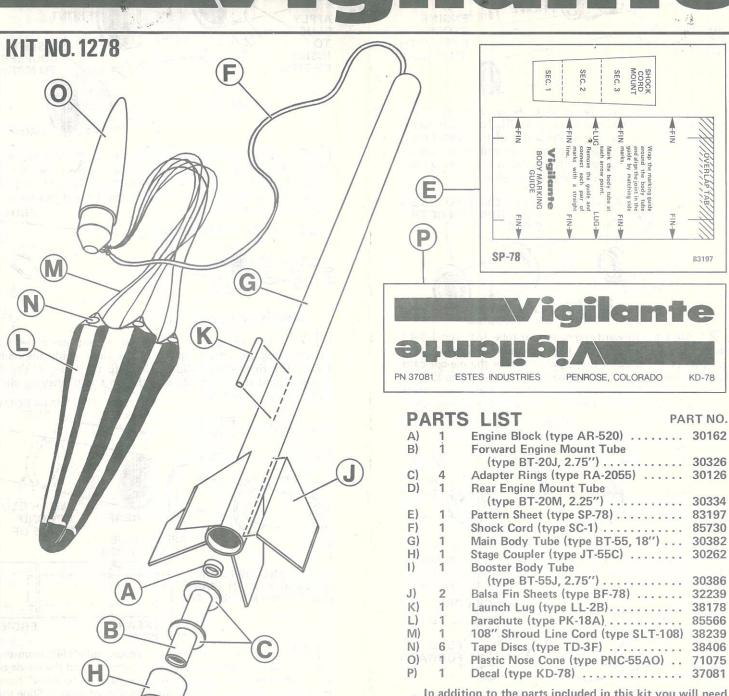
In addition to the parts included in this kit you will need scissors, white glue, a sharp model knife (or single edge razor blade), a pencil, a ruler, sandpaper, sanding sealer, and paint.
