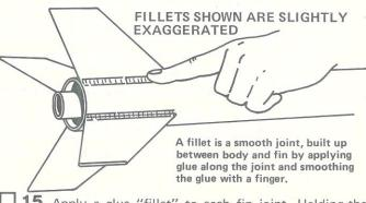
15 Apply a glue "fillet" to each fin joint. Holding the rocket horizontally (level), apply a line of glue to both sides of each joint. Smooth out the glue with your finger. Keep the rocket level until the grue dries.
