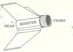
12 Rub a line of glue into the root edge of each fin and allow to dry. Glue the fins to the main body and the booster body on the fin alignment lines drawn in step 10. Refer to the illustration to be sure you position the fins correctly. The rear edge of each fin should be even with the rear edge of the body tube. Adjust the fins so they project straight away from the body tube. Do not set the rocket on its fins while the glue is wet.
