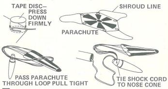
14 Cut out the parachute (part L) on its edge lines. Cut three 36" lengths of shroud line (part M). Attach line ends to the top of the parachute with tape discs (part N) as shown. Pass the shroud line loops through the ring on the nose cone (part O). Pass the parachute through the loop ends and draw the lines tight against the ring. Set knot with a drop of glue. Tie the free end of the shock cord to the nose cone ring.
