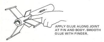
15 When the fin joints have dried, apply glue reinforcements to each main fin joint. Holding the fin mount assembly level, apply a narrow line of glue to both sides of each fin joint. Smooth out the glue with your finger. Keep the fin assembly level until the glue dries.
