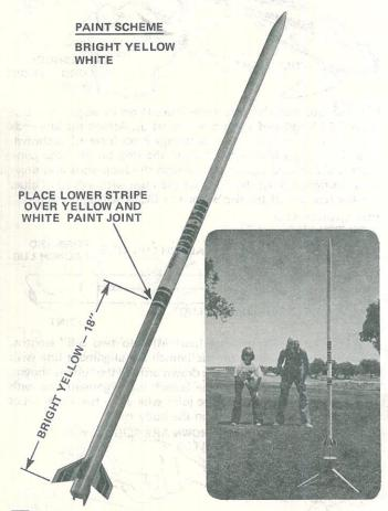
18 When all the paint is dry, apply decals (part N). Cut out a decal section, dip it in lukewarm water for about 15 seconds, and hold it until it uncurls. Slip the decal off the backing sheet and onto the model in the location shown in the illustration. Blot away excess water. For best results, let the model dry overnight and apply a coat of clear spray to protect the decals.
