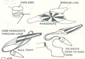
13 Cut out the parachute (part I) on its edge lines. Cut three 36" lengths of shroud line (part J). Attach the line ends to the top of the parachute with tape discs (part K) as shown. Pass the shroud line loops through the ring on the nose cone (part L). Pass the parachute through the loop ends and draw the lines tight against the ring. Set the knot with a drop of glue. Tie the free end of the shock cord to the nose cone.
