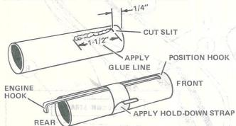
1 Cut a 1/8" wide slit in the engine mount tube (part A), 1/4" from one end as shown. Cut out the hold-down strap from the pattern sheet (part B). Apply a 1-1/2" long line of glue to the tube as shown. Push one end of the engine hook (part C) into the slit and press the main part of the hook into the glue. Apply glue to one side of the hold-down strap, and wrap it tightly around the middle of the tube over the engine hook.
