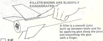
Reinforce the fin joints with glue. Holding the rocket horizontally (level), apply a line of glue to both sides of each joint. Smooth out the glue with your finger. Keep the rocket level until the glue dries.
