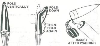
Loosely fold the parachute. Lay it on top of the wadding, with its shroud lines and shock cord on top of it. Slide the nose cone into place.
