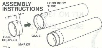
Mark the tube coupler (part L) in the middle (1/2" from one end). Put 3 or 4 marks around coupler so it can be positioned straight in the body tube. Run a bead of glue around the inside of one end of one 9" long body tube (part K). Push the coupler into the tube until the marks on the coupler line up with the end of the tube. Wipe away excess glue and set aside to dry.
