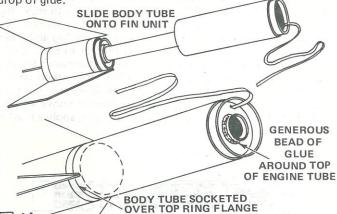
11 Slide the body tube assembly onto the fin unit. The bottom of the body tube should be socketed over the upper section of the fin ring and the engine tube should extend through the die-cut ring at the top of the body. Make sure the whole unit is pushed tightly together, then apply a generous bead of glue to the engine tube where it protrudes through the die-cut ring. Set the assembly aside and do not disturb until glue is completely set.
