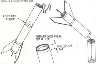
12 After the glue has dried on the main rocket assembly, attach the remaining body tube. Test fit the tube on top the assembly. If necessary, lightly sand the inside edge of the tube
