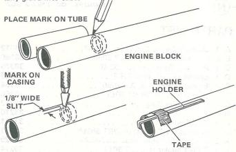
The engine holder is attached to the engine tube with one of its hooked ends against the engine block. To locate, hold the casing against the outside of the engine tube with the mark on the casing even with the end of the tube. Place a mark on the tube even with the top of the casing. Cut a 1/8" wide slit in the tube on the pencil mark. Insert one end of the engine holder into slit. Align holder with tube and temporarily secure with a piece of masking tape around bottom of tube.
