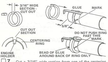
**7** Cut a 3/16" wide section from one of the centering rings (part B). Place a mark on the engine tube 5/8" from end. Apply a bead of glue around tube in rear of mark. Don't get
