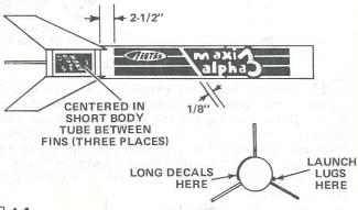
14 Apply the decals in the positions shown. Note that the long decal (in two pieces) is centered above the two fins opposite the side to which the launch lugs are attached. To apply decals, cut out individual decal, dip in water for 20-30 seconds (until decal slides off backing). Slide decal from backing paper onto desired surface. Blot dry with a clean damp cloth.
