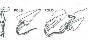
Gather the parachute as shown, then fold into a triangular shape. Fold again and insert into rocket body.
