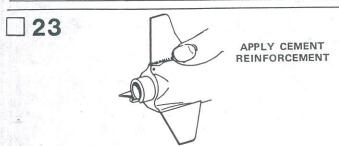
After all cement has dried, give each fin and rudder joint a plastic cement reinforcement. Hold model level and apply a line of tube-type plastic cement to both sides of each fin joint. Rub cement into missile body/fin joint and smooth out the cement with your finger. Keep the model level until cement dries.
