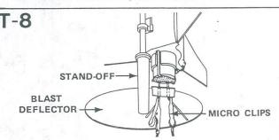
Slide launch rod through rocket launch lugs and place rocket on launch pad. Make sure the rocket slides freely on launch rod. Clean the micro-clips and attach them to the igniter wires. Arrange the clips so they do not touch each other or the metal blast deflector. Attach clips as close to engine as possible.
