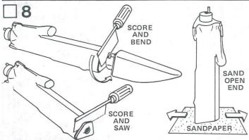
Lightly score around the nose cone/body joint with a razor saw on the Cruise Missile body (part H). Bend body gently so it breaks apart at the scored line. Using the razor saw cut the missile body along the edge of the shoulder and missile body as shown. Lay a sheet of sandpaper flat on your work surface and pass the open end of the body across it to smooth out the edges. Be careful not to sand off too much of the plastic.
