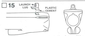
Remove the launch lug from the plastic hinge/lug set. Using tubetype plastic cement smear a small amount on the bottom side of the launch lug. Make sure the hold down tab for the wings is pointing forward as shown. Cement the lug to the rear lug mount on the missile body. Make sure the lug is aligned over the rear lug mount on the missile body.
