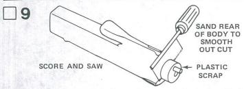
Score around the missile body at the rear of the body with the razor saw and then carefully cut along the scored line with the razor saw to remove the scrap end of plastic. The blow-molded plastic is thicker here, and requires care and patience to cut.
