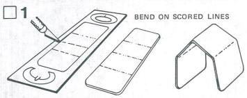
Carefully remove the parachute tube support from the die-cut card (part A). Use a modeling knife to free the part from the sheet. Bend it on the scored lines to the shape shown.
