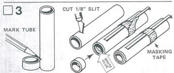
Stand the engine tube (part C) next to the engine block (part D), and mark the engine tube with a pencil as shown. Make a 1/8" slit in the engine tube at the pencil mark. Push the engine hook (part E) into the slit and apply a piece of masking tape to hold hook in place as shown. Run a bead of glue around inside of the slit end of the engine tube. Insert the engine block as shown. Make sure engine block is against engine hook.
