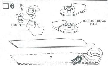
Remove the wing hinge halves from the plastic hinge/lug set (pg. G). Carefully sand the hinge part that goes inside the other half until the assembled parts rotate easily, but do not sand so much as to cause them to be too loose. Pull the two pieces apart and cement a wing hinge half to each wing with tube-type plastic cement, making sure the wing fits correctly into the area provided in the wing hinge half as shown. Allow these parts to dry thoroughly.
