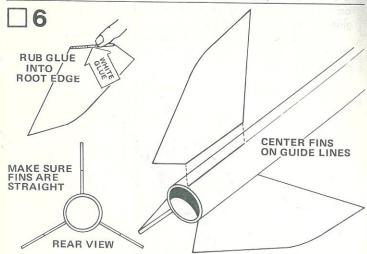
Rub glue into the root edge of each fin and allow to dry. Apply glue to the fins again and position fins on the alignment lines in positions shown. Adjust the fins so they project straight away from the body tube. DO NOT set the rocket on its fins while the glue is wet.
