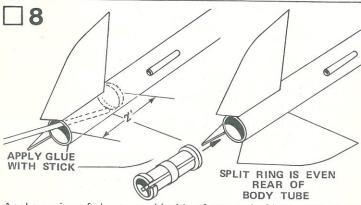
Apply a ring of glue around inside of rear end of body tube about 2" to 2-1/2" form the end of the tybe. Apply with a stick or dowel as shown. Immediately insert the engine mount unit, being careful
