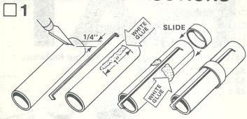
Cut a 1/8" slit in the engine mount tube (part A), 1/4" from one end as shown. Apply a 1" long line of glue to the tube. Push one end of the engine hook (part B) into the slit and press the main part of the hook into the glue. Apply a line of glue around the middle of the tube and slide the hook retainer ring (part C) over tube and hook, onto the glue.
