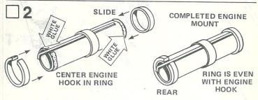
Glue the split centering ring (part D) to the engine mount tube so the engine hook is centered in slot in ring and even with rear of tube. Avoid getting glue into the slot. Glue the other ring (part E) to the front of the engine tube against the end of the hook as shown.
