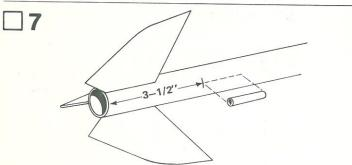
Glue launch lug (part I) to rocket body tube on the launch lug line. The rear of the launch lug should be 3-1/2" from the rear of the rocket body tube. Align the launch lug straight along the body.
