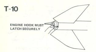
Insert engine into rocket engine mount. Engine hook must latch securely over end of the engine.
