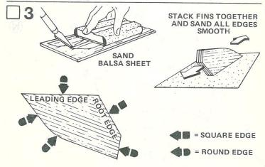
Fine-sand the balsa die-cut sheet (part F). Free the edges with a sharp knife then carefully remove the die-cut fins from the sheet. Sand the leading and trailing edges of the fins round. Leave edge designated root edge square.
