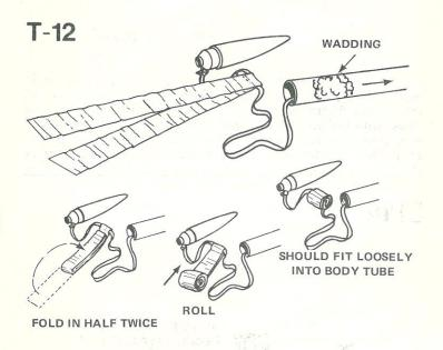
Fold the streamer in half lengthwise. Fold again, then roll until the streamer fits loosely into the rocket body. Pack the shock cord neatly into the rocket body. Slide nose cone into place.
