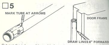
Cut out the tube marking guide from the pattern sheet (part G) and wrap it around the body tube (part H). Mark the body tube at each of the arrow points. Draw straight lines connecting each mark. A door frame inside edge can be used as a guide as shown. Extend the lines about 6" forward from the rear of the tube.
