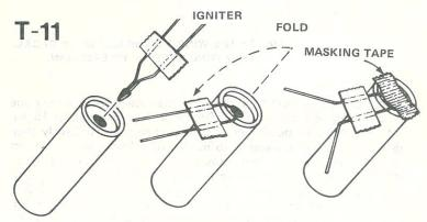
Select an engine and install an igniter as directed in the engine instructions. Use an A8-3 engine for your first flight.
