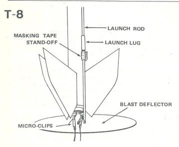
Slide launch rod through rocket launch lug and place rocket on launch pad. Make sure the rockt slides freely on the launch rod. Clean the micro-clips and attach them to the igniter wires. Arrange the clips so they do not touch each other or the metal blast deflector. Attach clips as close to engine as possible.
