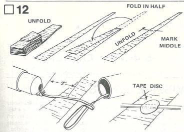
Tie the free end of the shock cord to the nose cone (part K). Unfold the streamer (part L) and fold lengthwise to find its center.
