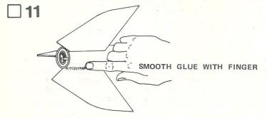
When the glue on the fin joints has dried, apply a glue reinforcement to each fin body tube joint. Holding the model level, apply a line of glue to both sides of each fin joint. Smooth out the glue with your finger. IMPORTANT -- Keep the model level until the glue dries.
