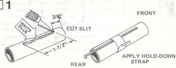
Cut a 1/8" wide slit in the engine mount tube (part A), 3/8" from one end as shown. Cut out the hold-down strap from the pattern sheet (part B). Apply a 1-1/2" long line of glue to the tube as shown. Push one end of the engine hook (part C) into the slit and press the main part of the hook into the glue. Apply glue to one side of the hold-down strap, and wrap it tightly around the middle of the tube over the engine hook.
