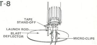
Slide launch rod through rocket launch lug and piace rocket on launch pad. Make sure the rocket slides freely on the launch rod. Clean the micro-clips and attach them to the igniter wires. Arrange the clips so they do not touch each other or the metal blast deflector. Attach clips as close to engine as possible.
