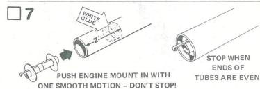
Smear glue around the inside of the rear end of the rocket body tube (part G) to cover an area about 2" from the end of the tube. Use a stick or dowel as shown. Immediately insert the engine mount being careful to position it so the end of the tubes are even and the hook projects out of the end of the body tube. Push engine mount in with one smooth motion.
