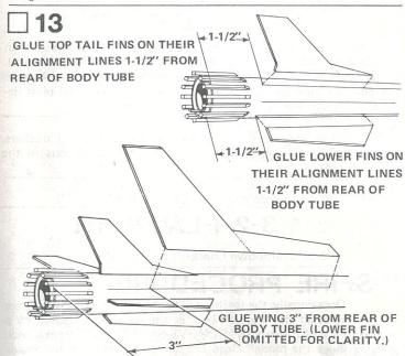
Rub a line of glue into the root edge of each fin and allow to dry. Apply glue to the fins and position fins on the alignment lines in their correct positions on the tube. Refer to the illustration to be sure of these positions. Adjust the fins so they project straight away from the body tube. Do not set the rocket on its fins while the glue is wet.
