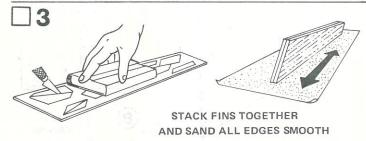
Fine-sand the balsa die-cut sheet (part E), then carefully remove the die-cut parts from the sheet by freeing the part edges with a sharp knife. Sand the edges of the fin parts slightly to remove any rough spots, but leave edges square and sharp.
