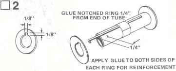
Separate the adapter rings from the die-cut card (part D). Cut a notch in one of the rings as illustrated and glue the rings to the engine mount tube. The notched ring should be placed over the engine hook. Let this assembly dry completely.
