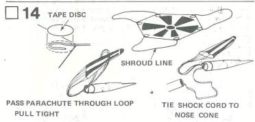
Cut out the parachute (part I) on its edge lines. Cut three 36" lengths of shroud line (part J). Attach the line ends to the top of the parachute with tape discs (part K) as shown. Pass the shroud line loops through the ring on the nose cone (part L). Pass the parachute through the loop ends and draw the lines tight against the ring. Set the knot with a drop of glue. Tie the free end of the shock cord to the nose cone.
