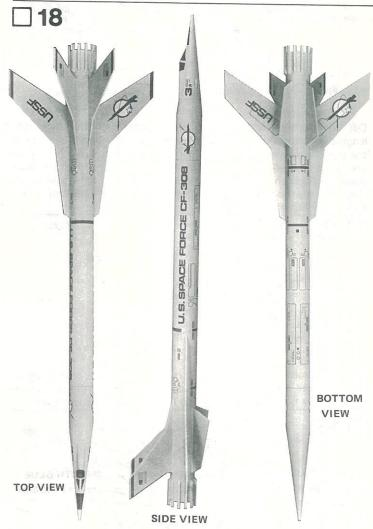
Apply the decals (part N) in the positions shown. Cut out a decal section, dip in lukewarm water for 10-20 seconds, and hold it until it starts to uncurl. Slip the decal off the backing sheet and onto the model. Blot excess water away. For best results, let model dry overnight and apply a coat of clear spray to protect the decals.
