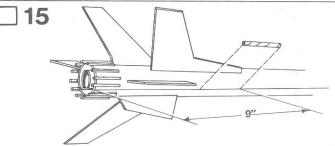
Glue the launch lug (part M) to rocket body tube on the launch lug line. The front of the lug should be 9" from the rear of the rocket body tube. Align the launch lug straight along the body.
