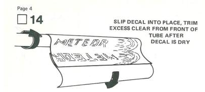
Apply the decal (part N) in the position shown. Cut out decal, dip in lukewarm water for 10-20 seconds, and hold it until it starts to uncurl. Slip decal onto front portion of rocket body tube and rotate rocket while slipping backing paper out from under decal. Match up ends of decal and blot away excess water. For best results, let the model dry overnight and apply a coat of clear spray to protect the decal.
