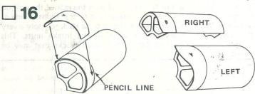
Cut shrouds A and B from the printed sheet and attach to the BT-60 units in a similar manner as you did in Step 14. Pre-curl the shrouds and glue to the tubes with the rear edge of the shrouds on the pencil lines (from Step 12). Note that there is a right unit and a left unit.
