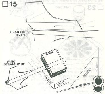
Proceed ONLY if the glue on the top fin is completely dry. Attach the left wing to the body using the same procedure as in Step 11.
