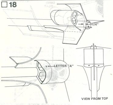
Mark the body 1/4" from the rear edge on both sides of the top fin. Run a bead of glue around the edges of left intake unit (letter
