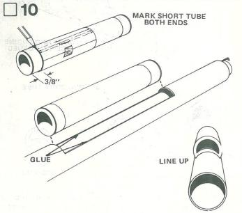
Mark the 5" body tube at a point 3/8" from EACH END. Wrap the marking guide around the tube and use one end as a guide to draw
