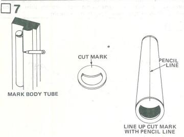
Place the 5" long body tube (part K) against a door jamb and draw a line along the length of the tube. Remove the two small rings from the die-cut card (part M). There is a small cut mark at the top of each ring. Glue the rings to the ends of the tube with the cut marks lined up with the pencil line.
