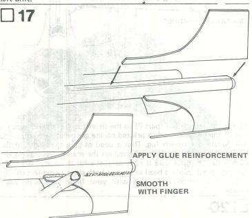
Proceed with this step only after the glue on the other wing is completely dry. Attach the remaining wing in the manner outlined in Steps 11 and 15. Allow the glue to dry completely, then apply glue reinforcements. Run a bead of glue along both sides of the top fin/body tube joint. Pull your finger along the joint, smoothing the glue. Remove any excess glue. Repeat with both wings.
