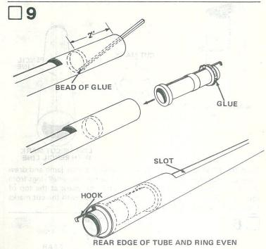
Use the stick to apply a generous bead of glue 2" inside the rear of the main body tube (this is the end with slot and pencil marks). DO NOT GLUE THE MOUNT INTO THE WRONG END OF THE BODY TUBE. Apply a light bead of glue to the rear (split) centering ring of the engine mount. Slide the mount into the tube with the engine hook and slot aligned. Push the mount in until the rear edges of the body tube and split centering ring are even. Wipe away excess glue.
