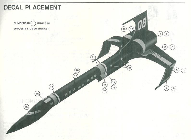
The decal sheet (part V) has numbers printed next to each decal. The decals should be applied in numerical order. Refer to the photograph for location of the decals. To apply decal, cut one decal at a time from the sheet. Submerge decal in water for 15 to 30 seconds (until decal slides on backing paper). Gently slide decal from backing paper onto model. Move decal into exact position and carefully blot away excess water with a soft cloth. If the decal
