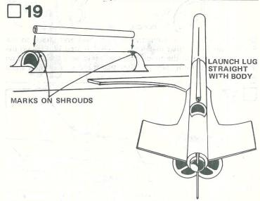
Attach the launch lug (part P) to the short tube on the underneath side of the body. A mark is printed on the center of each shroud to help locate the launch lug. Run a bead of glue the length of the lug and attach to the tube aligned on the marks. Sight along the launch lug to make sure it runs parallel with the body. After the glue has dried, apply a bead of glue to both sides of the launch lug/body joint. Smooth the glue with your finger and wipe away excess.
