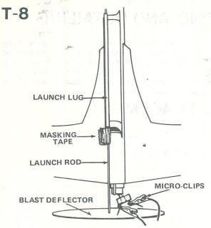
Slide the launch lug of the rocket onto the launch rod. Make sure the rocket slides freely on the launch rod. If the launch pad you are using does not have a deflector stand-off, place a piece of masking tape on the rod as shown to keep the rocket 2" above the deflector. Clean the micro-clips and attach them to the igniter wires as close to the tape as possible. Arrange the clips so they do not touch each other or the metal blast deflector.
