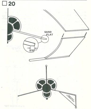
Sand a flat on the bottom side of each wing as shown. Cut the wing/finlet alignment guide from the pattern sheet. Apply a bead of glue to the root edge of one finlet, attach to wing, then remove.
