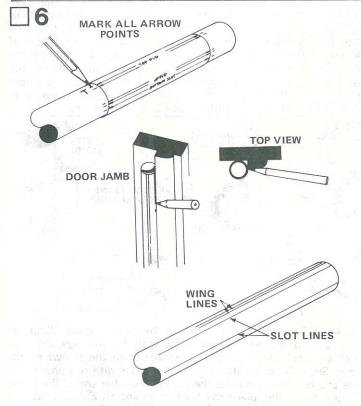
Cut the BT-50 body tube marking guide from the pattern sheet (part I). Wrap the guide around the main body tube (part J) about
