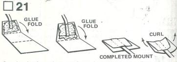
Cut the shock cord mount from the pattern sheet. Fold on dotted lines, then unfold and apply glue to Section 1. Lay the end of the shock cord (part Q) into the glue. Fold over and apply glue to the back of Section 1 and the exposed portion of Section 2. Fold again to complete mount. Curl the edges of the mount up so it will match the contour of the body tube and hold with your fingers until the glue sets.
