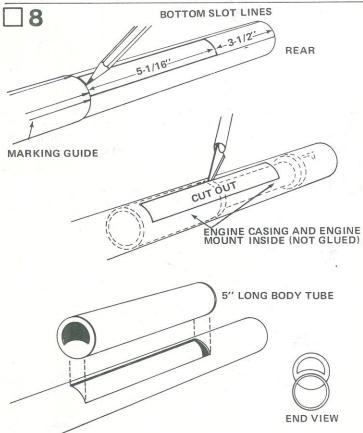
The object of this step is to cut a slot in the main body tube so that the 5" long body tube will nest partially into the main tube. Study the drawings before beginning.
