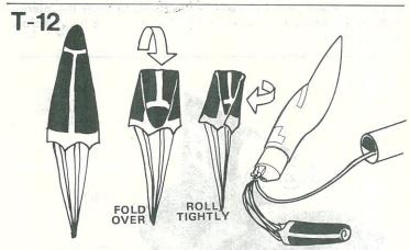
Hold the parachute at its center and pass the other hand down it to form a "spike" shape. Fold this spike in half. Roll parachute into tube shape to fit easily into body. Pack 'chute into the tube on top of the wadding. Pack the shroud lines and shock cord in on top of the parachute and slip the nose cone into place.
