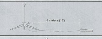
6 Insert safety key to arm the launch controller.
