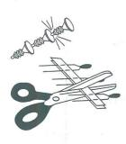
A. Separate igniter and igniter plug.
