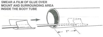
Use a stick or scrap dowel to apply a generous amount of glue inside the body tube 1" from the front of the tube. Slide the shock cord mount into the tube and press it into the glue. To insure a good bond use a stick or your finger to smear a film of glue over the mount and surrounding area in the body tube.
