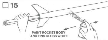
When all glue on the outside of the body is dry, insert a sheet of rolledup newspaper or heavy paper into rear of rocket body as shown. <u>THE PAPER MUST FIT TIGHTLY</u>. Apply two or three light coats of gloss white spray enamel to the model. Allow each coat of paint to dry completely.
