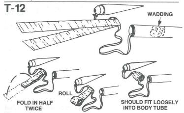
Fold the streamer in half lengthwise. Fold again, then roll until the streamer and shock cord fit loosely into the rocket body. Slide the nose cone into place.
