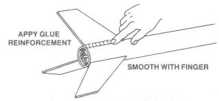
Apply glue reinforcements to each fin/body tube joint. Holding the model level, apply a narrow line of glue to both sides of each fin joint. Smooth out the glue with your finger. Apply glue reinforcement on both sides of launch lug. IMPORTANT -- Keep the model level until the glue dries.
