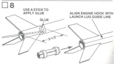
Apply a ring of glue around inside of rear end of body tube about 2" to 2-1/2" from the end of the tube. Use a stick or dowel as shown. Immediately insert the engine mount unit, being careful to position it so the engine hook will stick out of the end of the tube. Push engine mount in with one smooth motion until the end of the engine mount tube and the end of the body tubes are even.
