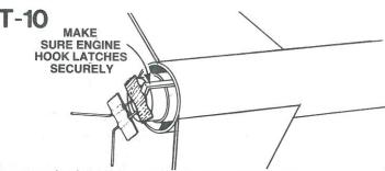
Insert engine into rocket engine mount. Engine hook must latch securely over end of the engine.
