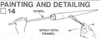
Spray paint the nose cone with several light coats of green paint. The nose cone can be supported by a dowel or stick inserted in the center opening in the nose cone while being painted and drying. A layer of masking tape around nose cone shoulder works well to protect the nose cone shoulder from "overspray" while painting.
