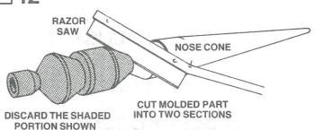
If you have a razor saw, use it to cut the molded nose-tail cone (part I) into two parts as shown. If you do not have a razor saw, use a model knife or single edge razor blade. Make very light cuts around the parting lines (bottom of grooves) and repeat until you have cut completely through the plastic. Work carefully to avoid tearing the plastic. Keep the nose cone and discard the rest of the plastic unit.
