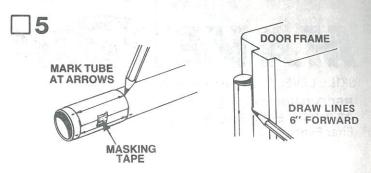
Cut out the tube-marking guide (part E) from the back of the display panel, and wrap it around the body tube (part F). Mark the body tube at each of the arrow points. Draw straight lines connecting each mark. A door frame inside edge can be used as a guide as shown. Extend the lines about 6" from the rear of the tube.
