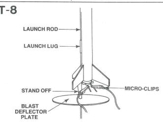
Slide launch rod through rocket launch lug and place rocket on launch pad. Make sure the rocket slides freely on the launch rod. Clean the micro-clips and attach them to the igniter wires. Arrange the clips so they do not touch each other or the metal blast deflector. Attach clips as close to protective tape on igniter as possible.
