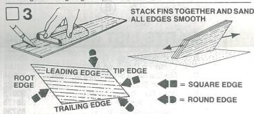
Fine-sand the balsa die-cut sheet (part D), then carefully remove the die-cut fins from the sheet. Free the edges with a sharp knife. Sand the leading and trailing edges of the fins round. Leave other edges square.
