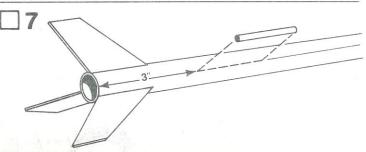
Glue launch lug (part G) to rocket body tube on the launch lug line. The rear of the launch lug should be 3" from the rear of the rocket body tube. Align the launch lug straight along the body.
