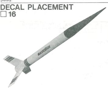
Apply the decals (part K) in the positions shown. Cut out decal, dip in lukewarm water for 10-20 seconds, and hold it until it starts to uncurl. Slip decals into proper positions while slipping backing paper out from under decal. Match up ends of decal and blot away excess water. For best results, let the model dry overnight and apply a coat of clear spray to protect the decal.
