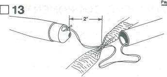
Using a double knot, tie the shock cord around the middle of the plastic streamer (part J) about 2" from the end of the shock cord. Attach the free end of the shock cord to the nose cone with a firm knot.
