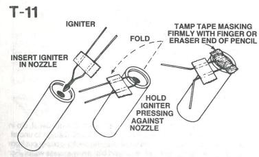
Select an engine and install an igniter as directed in the engine instructions. Use an A8-3 engine for your first flight.
