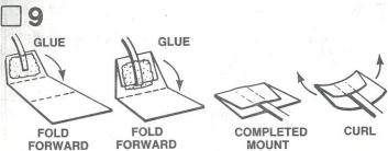
Cut out the shock cord mount from the front page of the instruction sheet. Crease it on the dotted lines by folding. Spread glue on the first section (1) and lay the end of the shock cord (part H) into the glue. Fold over and apply glue to the back of the first section and the exposed part of section 2. Lay the shock cord as shown and fold over again. Clamp the unit together with your fingers until the glue sets.
