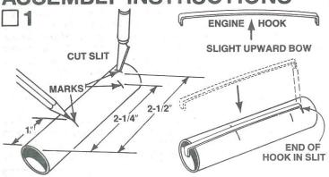
Mark the engine mount tube (part A) at 1", 2-1/4", and 2-1/2" from one end. Cut a 1/8" long slit at the 2-1/2" mark. Gently bend the engine hook (part B) so that it bows upward very slightly in the middle. (Study the drawing — Don't bend the wrong way.) Insert one end of the engine hook into the slit in the tube.
