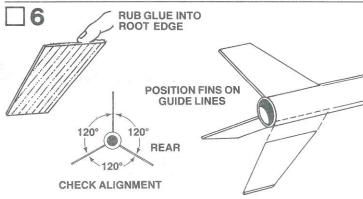
Rub a line of glue into the root edge of each fin and allow to dry. Apply glue to the fins and position fins on the alignment lines in their correct positions on the tube. Refer to the illustration to be sure of these positions. Adjust the fins so they project straight away from the body tube. Do not set the rocket on its fins while the glue is wet.
