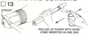
Trim away the excess plastic from the nose cone eyelet and from around the nose cone (part H). Spray paint the nose cone with several light coats of dark blue spray paint. The nose cone can be supported by wrapping newspaper around the shoulder of the nose cone and securing it with masking tape.
