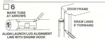
Cut out the tube marking guide from the front of the instructions and wrap it around the body tube. Place the tube marking guide so that the engine hook will line up with the launch lug placement line (arrow point). Mark the body tube at each of the arrow points. Draw straight lines connecting each pair of marks. A door frame inside edge can be used as a guide as shown. Extend the lines about 6" forward from the rear of the tube.
