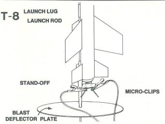
Slide the launch rod through rocket launch lug and place rocket on launch pad. Make sure the rocket slides freely on the launch rod. Clean the micro-clips and attach them to the igniter wires. Arrange the clips so they do not touch each other or the metal blast deflector. Attach clips as close to protective tape on igniter as possible.
