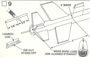
Cut the launch lug (part F) into two 5/8" lengths. Glue the two lugs to the two balsa launch lug stand-offs as shown. Make sure they are glued straight. Then glue these lug assemblies to the body tube on the launch lug line. The rear stand-off should be glued even with the rear of the body tube. The forward stand-off is glued to the body 4" from the rear of the tube. Sight down the body tube to be sure the lugs are straight before the glue sets.
