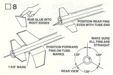
Rub glue into the root edge of each fin and allow to dry. Apply glue to the fins again and position fins on the alignment lines in positions shown. Adjust the fins so they project straight away from the body tube. DO NOT set the rocket on its fins while the glue is wet.
