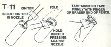
Select an engine and install an igniter as directed in the engine instructions. The engines recommended for use with this rocket are the A8-3, B4-4, B6-4, B8-5 and C6-5 made by Estes . Use an A8-3 for your first flight.
