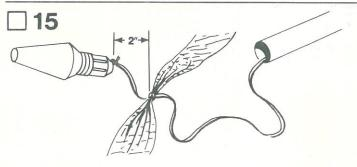
Using a double knot, tie the shock cord around the middle of the plastic streamer (part I) about 2" from the end of the shock cord. Attach the free end of the shock cord to the nose cone with a firm knot.
