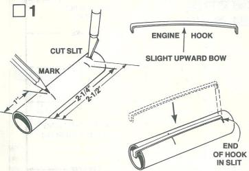
Mark the engine mount tube (part A) at 1", 2-1/4" and 2-1/2" from one end. Cut a 1/8" wide slit at the 2-1/2" mark. Gently bend the engine hook (part B) so that it bows upward very slightly in the middle. (Study the drawing—Don't bend the wrong way.) Insert one end of the engine hook into the slit in the tube.
