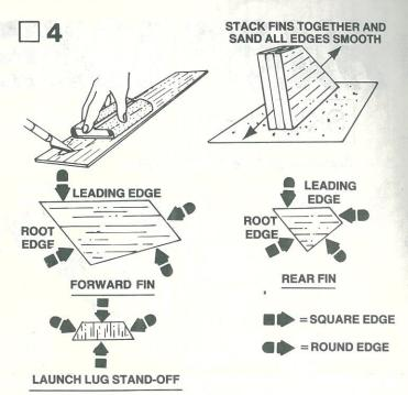
Fine sand the balsa die-cut sheet (part E), then carefully remove the die-cut fins from the sheet. Free the edges with a sharp knife. Sand the leading and trailing edges of the fins round. Leave other edges square.
