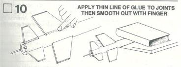
When the glue on the fin joints has dried, apply a glue reinforcement to each fin/body tube joint. Holding the model level, apply a line of glue to both sides of each fin joint and on both sides of the launch lug/stand-off. Smooth out the glue with your finger. IMPORTANT: Support rocket on the table edge as shown until the glue dries.
