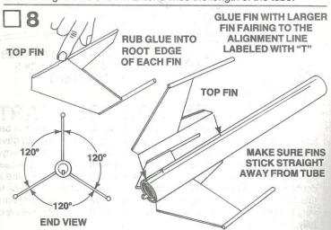
Rub a line of glue into the root edge of each fin and allow to dry. Apply glue to the fins again and position fins on the alignment lines in their correct positions on the tube. Glue top fin with the larger top fin fairing to the alignment line labeled with a "T". Refer to the illustration to be sure of these positions. Adjust the fins so they project straight away from the body tube. Do not set the rocket on its fins while the glue is wet.
