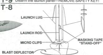
Slide the launch rod through rocket launch lug and place rocket on launch pad. Make sure the rocket slides freely on the launch rod. Clean the micro-clips and attach them to the igniter wires. Arrange the clips so they do not touch each other or the metal blast deflector. Attach clips as close to protective tape on igniter as possible.
