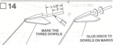
Remove the six discs from the die-cut card (part I). Use a sharp knife to free the parts from the card. Mark dowels as shown. Glue the discs to dowels on marks. Set assembly aside to dry.
