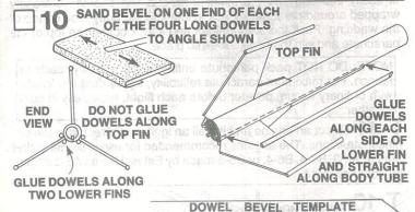
Locate the four 8-1/2" lengths of wood dowel from step 5. Sand a bevel on one end of each dowel to the angle shown. Glue the dowels, one on each side of the two lower fins, straight along the body tube. <u>Do not glue dowels along the top fin.</u>
