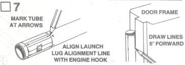
Cut out the body tube marking guide from the pattern sheet (part G) and wrap it around the body tube. Place the tube marking guide so that the engine hook will line up with the launch lug placement line (arrow point). Print the letter "T" next to the top fin marks for later identification. Mark the body tube at each of the arrow points. Draw straight lines connecting each pair of marks. A door frame inside edge can be used as a guide as shown. Extend lines the length of the tube.
