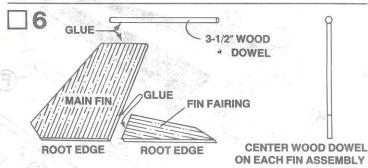
Assemble the fins as shown over a piece of waxed paper. Apply glue to edge of main fin and fin fairing as shown. Let glue partially dry. Apply second bead of glue to one edge and press parts together. Wipe away any excess glue. Repeat procedure for other two fin assemblies. Apply glue to a 3-1/2" dowel and position on top of each fin assembly as shown.
