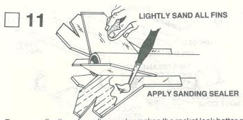
Proper application of sanding sealer makes the rocket look better and reduces drag so that the rocket will fly higher. However, this step is not essential to make a safe, attractive rocket. Apply a coat of sanding sealer to each fin. When sealer is dry, lightly sand all the sealed surfaces. Repeat sealing and sanding process until balsa grain no longer shows.
