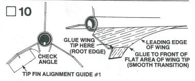
Cut out the tip fin alignment guide #1 (part H) found on the panel back. Lightly sand the root edge of two of the tip fins until they match the angle of the tip fin alignment guide #1. See above illustration. Glue the tip fins to the wing tips so their leading edges are at the very front of the flat area of the wing tips. They should form a smooth transition with the curved leading edge of the wings. Check the angles of the tip fins again and set the assembly aside to dry.
