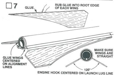
Rub glue into the root edge of each wing and allow to dry. Apply glue to the wings again and position wings on the alignment lines in positions shown. Adjust the wings so they project straight away from the body tube. DO NOT set the rocket on its wings while the glue is wet.
