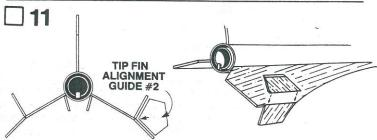
Cut out the tip fin alignment guide #2 (part I) found on the panel back. Glue the remaining two tip fins on the top of the wings so they are even with the tip fins installed in step #10. See above illustration for correct location. Use the tip fin alignment guide #2 to check for proper angles. Allow these fins to dry completely.
