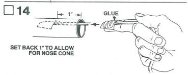
Apply glue to the back of the shock cord mount. With the shock cord mount positioned on the end of your finger, gently position mount down into front of body tube far enough from the front edge of the tube to allow for the nose cone to fit into place. Press shock cord mount firmly into position. To insure a good bond, smear a film of glue over the mount and surrounding area in the body tube.
