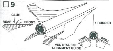
Cut the ventral fin alignment guide (part G) from the back of the kit panel. Repeat the gluing procedure for the two ventral fins and glue them to the undersides of the wings even with the rear end of the body tube, and along the wing/body tube joints. Use the ventral fin alignment guide to get these fins at the proper angle to the wing bottoms. Allow the ventral fins to dry completely.
