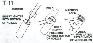
Select an engine and install an igniter as directed in the engine instructions. The engines recommended for use with this rocket are the A8-3, B4-4, B6-4, B8-5, C6-5, and C6-7 made by Estes.
