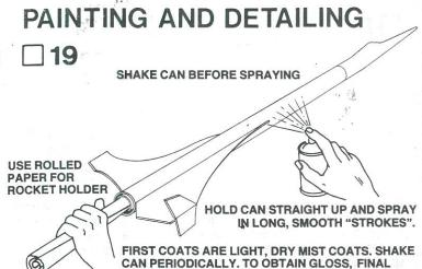
After the sanding sealer is completely dry, paint the entire model Krylon "True Blue". Follow instructions on spray can for best results. We recommend spray enamel. Do not paint the model with lacquer paint. Lacquer will mar the finish of the plastic nose cone. Spray the model with several light coats of paint to avoid "runs". Let this coat dry overnight.
