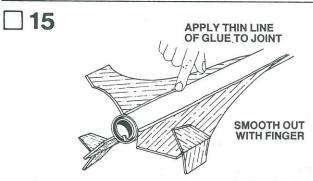
When the glue on the fin joints has dried, apply a glue reinforcement to each fin/body tube joint. Holding the model level, apply a line of glue to both sides of each balsa joint and on both sides of the launch lug. Smooth out the glue with your finger. IMPORTANT—Keep the model level until the glue dries.
