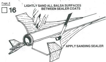
Proper application of sanding sealer makes the rocket look better and reduces drag so that the rocket will fly higher. However, this step is not essential to make a safe, attractive rocket. Apply a coat of sanding sealer to each wing and the rudder. When sealer is dry, lightly sand all the sealed surfaces. Repeat sealing and sanding process until balsa grain no longer shows.
