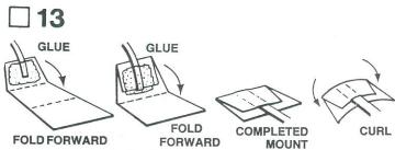
Cut out the shock cord mount (part K) found on page 1 of instructions. Fold on dotted lines, then unfold and apply glue to Section 1. Lay the end of the shock cord (part L) into the glue. Fold over and apply glue to the back of Section 1 and the exposed portion of Section 2. Fold again to complete mount. Curl the edges of the mount down so it will match the contour of the body tube and hold with your fingers until the glue sets.
