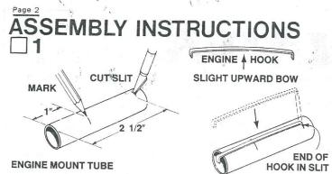
Mark the engine mount tube (part A) at 1" and  $2^{1/2}$ " from one end. Cut a 1/8"long slit at the  $2^{1/2}$ " mark. Gently bend the engine hook (part B) so that it bows upward very slightly in the middle. (Study the drawing—Don't bend the wrong way.) Insert one end of the engine hook into the slit in the tube.
