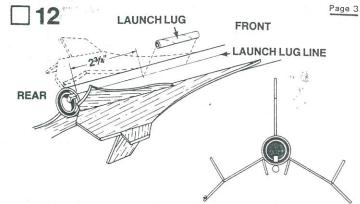
Turn model over and measure 29/4" from the rear of the model up the launch lug line and make a mark. Glue the rear end of the launch lug (part J) to the launch lug line at the 29/4" mark as shown in the illustration. Be sure the launch lug is centered on the launch lug line.
