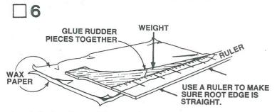
Locate the two pieces of the rudder taken from the die-cut balsa sheet in step 5. Place glue on one of the two matching edges as shown in step 5. Join the two pieces on a piece of wax paper. Use a ruler to be sure the root edge is straight. Now place another piece of wax paper over the assembly and put a book or other weight on the assembly. Allow the rudder to dry completely.
