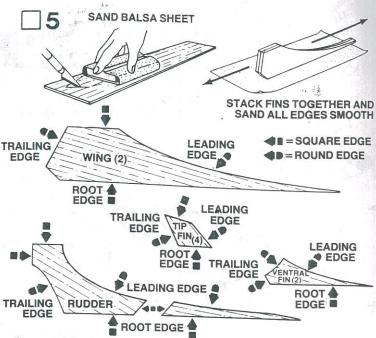
Fine-sand the balsa die-cut sheet (part F). Free the fin edges with a sharp knife, then carefully remove the die-cut fins from the sheet. Stack each group of fins together as shown and sand all four sides as illustrated. Lightly sand both sides of each fin. Sand the leading edge, tip edge, and trailing edge of each fin round or square as shown. Leave the root (body) edge sanded "flat". The root edge may be identified by careful comparison with the drawings.
