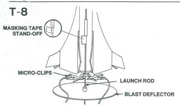
Slide the launch rod through rocket launch lug and place rocket on launch pad. Make sure the rocket slides freely on the launch rod. Clean the micro-clips and attach them to the igniter wires. Arrange the clips so they do not touch each other or the metal blast deflector. Attach clips as close to protective tape on igniter as possible.
