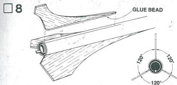
Rub glue into the root edge of the completed rudder assembly from step #6 and allow to dry. Apply glue to the rudder again and position it on the alignment line opposite the engine hook as shown. Adjust the rudder so it projects straight away from the body tube and is equally spaced between the wings. Do not set the rocket on its wings or rudder while the glue dries.
