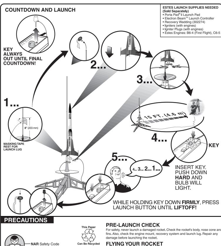
For safety, never launch a damaged rocket. Check the rocket's body, nose cone and fins. Also, check the engine mount, recovery system and launch lug. Repair any damage before launching the rocket.
