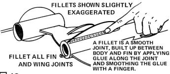
☐ 16 Apply a glue fillet to each fin and wing joint. Holding the rocket horizontally (level), apply a line of glue to both sides of each fin joint. Smooth out the glue with your finger. Keep the rocket level until the glue dries.
