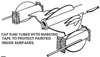
L 18 Give the entire rocket a spray base coat of white enamel (it may be easier to use brush-on enamel for the insides of the ram tubes only). When the base coat is dry, paint the insides of the ram tubes bright fluorescent orange. Cap the ends of the ram tubes with masking tape. Paint the outside of the rocket using a light color (yellow or orange) for the forward body-from the front fin forward including nose cone. Use black for the remaining rear section of the rocket.
