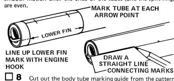
Cut out the body tube marking guide from the pattern sheet. Wrap it around the rear of the body so the lower fin mark is in line with the engine hook. Mark the tube at each arrow point, front and rear. Draw a straight line connecting each matching front and rear mark (use a ruler when drawing lines). Extend the wing lines forward 7". Extend the launch lug lines forward 5".
