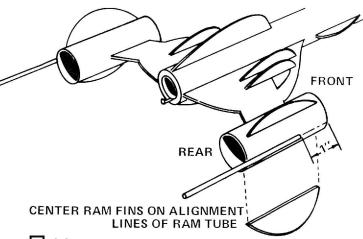
14 Carefully remove the ram tube fins from the balsa sheet. Glue the ram fins to the ram tubes on the alignment lines, positioning them so they are centered on the tube. Cut the dowel (part K) into two pieces, each 3-3/4" long. Glue the dowels to the ram tubes on the alignment lines so the front of each dowel is 1" from the front of its tube.
