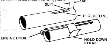
Mark the engine mount tube (part C) 1/4" from one end. Cut a 1/8" long slit in the tube at the mark as shown. Cut out the hold-down strap from the pattern sheet. Apply a 1" long line of glue to the tube as shown. Push one end of the engine hook (part D) into the slit and press the main part of the hook into the glue. Apply glue to one side of the hold-down strap and wrap it tightly around the middle of the tube over the engine hook.
