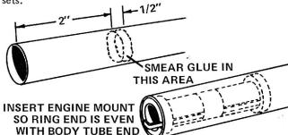
Install the engine mount assembly in the end of the body tube opposite the shock cord mount. Smear glue around the inside of the body tube to cover an area about 2" to 2-1/2" from the end of the tube. Immediately insert the engine mount unit, being careful to position it so the engine hook will stick out of the end of the tube. Push the engine mount in with one smooth motion until the ends of the tubes (and the split ring) are even.
