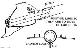
12 Glue the launch lugs (part J) to the body. The front of each lug should be 5" from the rear of the body tube. Position the lugs so they are to each side of the bottom fin as shown.
