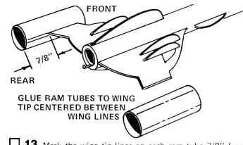
13 Mark the wing tip lines on each ram tube 7/8" from one end. Glue the ram tubes to the wing tips, centered between the wing lines, so the rear of each tube is 7/8" from the rear of the wing tip.
