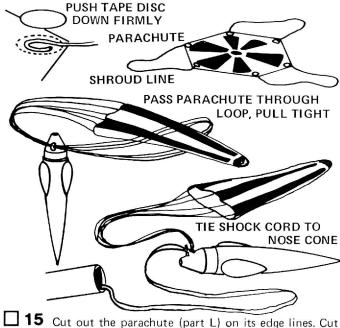
L 15 Cut out the parachute (part L) on its edge lines. Cut three 24" lengths of shroud line (part M). Attach line ends to the top of the parachute with tape discs (part N) as shown. Pass the shroud line loops through the ring on the nose cone (part O). Pass the parachute throught the loop ends and draw the lines tight against the ring. Set the knot with a drop of glue. Tie the free end of the shock cord to the nose cone ring.
