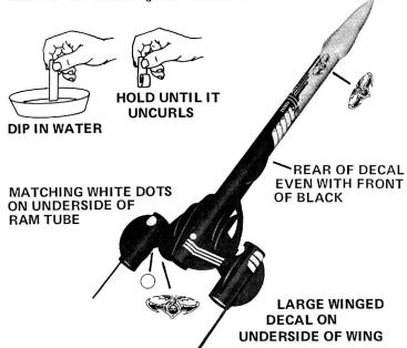
☐ 19 When all paint is dry, apply decals (part P) as shown in the photo. Cut out a decal section, dip it in lukewarm water for 10 seconds, and hold it until it uncurls. Slip the decal off the backing sheet and onto the model. Blot excess water away. For best results, let the model dry overnight and apply a coat of clear spray to protect the decals.
