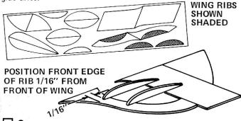
Carefully remove the wing ribs from the balsa sheets. Sand their edges smooth, then apply glue and position them on the wings in the positions shown in the assembly patterns. The front of each rib should be 1/16" from the front of the wing. Be careful to not disturb the wing panels.
