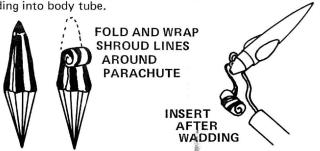
**T-13** Fold the parachute into a triảngular shape. Roll 'chute tightly as shown and wrap shroud lines around it. If 'chute is too large, unroll it and repack until it slides easily into rocket. A fit that is too tight may prevent parachute from ejecting properly.
