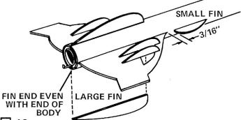
10 Carefully remove the body fins from the balsa sheet and sand their edges smooth. Glue the two large fins to the body, centered on the alignment lines, so their smaller ends are even with the rear of the body. Glue the two small fins to the body, exactly in line with the wings, 3/16" ahead of the wings. The small end of these fins should point forward.
