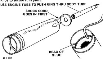
Locate the body tube and coupler which you glued together in step 1. Apply a bead of glue around the inside of the body tube at the base of the coupler. Insert the die-cut ring into the opposite end of the body tube with the shock cord extending through the body first (as shown). Use the engine tube to push the ring through the body-tube until the ring is tight against the bottom of the coupler. Apply a second bead of glue around the ring-coupler joint and set aside to dry.
