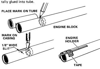
The engine holder is attached to the engine tube with one of its hooked ends against the engine block. To locate, hold the casing against the outside of the engine tube with the mark on the casing even with the end of the tube. Place a mark on the tube even with the top of the casing. Cut a 1/8" wide slit in the tube on the pencil mark. Insert one end of the engine holder into slit. Align holder with tube and temporarily secure with a piece of masking tape around bottom of tube.
