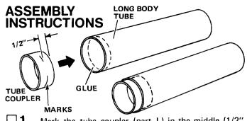
1 Mark the tube coupler (part L) in the middle (1/2" from one end). Put 3 or 4 marks around coupler so it can be positioned straight in the body tube. Run a bead of glue around the inside of one end of one 9" long body tube (part K). Push the coupler into the tube until the marks on the coupler line up with the end of the tube. Wipe away excess glue and set aside to dry.
