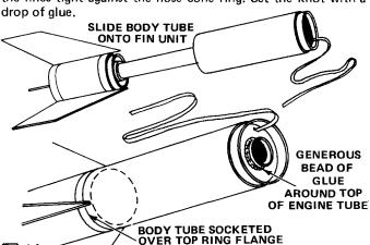
11 Slide the body tube assembly onto the fin unit. The bottom of the body tube should be socketed over the upper section of the fin ring and the engine tube should extend through the die-cut ring at the top of the body. Make sure the whole unit is pushed tightly together, then apply a generous bead of glue to the engine tube where it protrudes through the die-cut ring. Set the assembly aside and do not disturb until glue is completely set.
