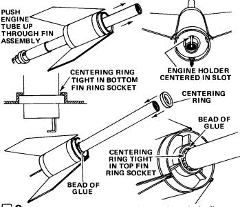
Slide the engine tube assembly up through the fin assembly as shown. Note that the engine holder must be centered
