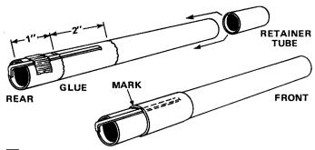
Place a mark on the engine tube 1" from the end. Smear a film of glue around the tube above this mark for a distance of 2". Make sure you have glue all around the upper portion of the engine holder. Slide the retainer tube onto the opposite end of the engine tube. Push the retainer down until it reaches the 1" mark. Wipe away excess glue.
