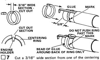
7 Cut a 3/16" wide section from one of the centering rings (part B). Place a mark on the engine tube 5/8" from end. Apply a bead of glue around tube in rear of mark. Don't get
