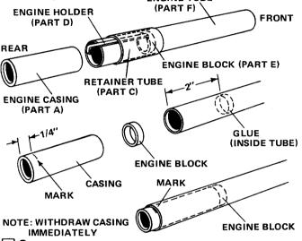
Locate the parts shown in the illustration. Place a mark on the engine casing 1/4" from one end. Using a small stick, apply a bead of glue inside one end of the engine tube approximately 2" from the end. Insert the engine block into this end of the tube and use the engine casing to push the block into place (with mark on casing even with end of engine tube). Withdraw casing immediately so it will not be accidentally glued into tube
