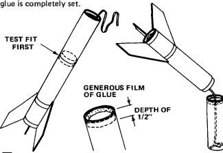
■ 12 After the glue has dried on the main rocket assembly, attach the remaining body tube. Test fit the tube on top the assembly. If necessary, lightly sand the inside edge of the tube
