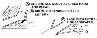
14 When all glue on the outside of the model is dry, prepare the balsa parts for painting. Apply at least two coats of sanding sealer to the fins. Let dry and sand lightly between coats. Do this until the tiny holes in the wood are filled and everything looks and feels smooth.
