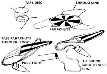
11 Cut out the parachute (part I) on its edge lines. Cut three 36" lengths of shroud line (part J). Attach the line ends
