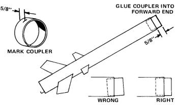
Mark the tube coupler (part H), 5/8" from one end. Smear a band of glue inside the finned body tube about 1/4" from the forward end. Insert the coupler and push until the mark on the coupler is even with the end of the tube. Be sure the tube coupler is installed squarely as shown.
