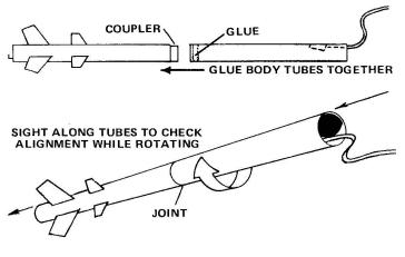
10 Smear a band of glue inside one end of the shock cord body tube about 1/4" from the end. Slide this end of the tube over the coupler attached to the finned tube in one smooth movement. The edges of the two body tubes should touch all around. Sight along the tubes while rotating the rocket to be sure the alignment of the body tubes is perfectly straight.
