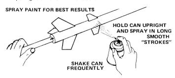
15 After the last coat of sanding sealer, sand again, then dust off the model. Paint the entire model gloss white. When the white paint is completely dry, paint the front part of the body tube (15" from rear of rocket) and nose cone a dark blue.
