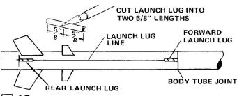
12 Cut the launch lug (part M) into two 5/8" lengths. Glue one of these lugs on the launch lug alignment line with its rear edge even with the line drawn around the tube as shown. Glue the remaining lug on the launch lug alignment line with its forward edge even with the joint where the two body tubes meet. Align the lugs straight on the body tube.
