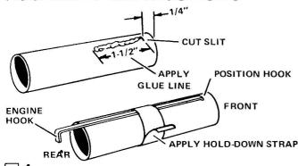
Cut a 1/8" wide slit in the engine mount tube (part A), 1/4" from one end as shown. Cut out the hold-down strap from the pattern sheet (part B). Apply a 1-1/2" long line of glue to the tube as shown. Push one end of the engine hook (part C) into the slit and press the main part of the hook into the glue. Apply glue to one side of the hold-down strap, and wrap it tightly around the middle of the tube over the engine hook.
