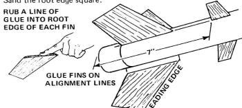
tube on the fin lines as shown. The rear of each large fin should be even with the line drawn 2" from the tube rear. Glue the small forward fins to the body tube on the fin lines. The rear of each small fin should be 7" from the rear of the body tube. Adjust all fins so they project straight away from the body tube. Do not set the rocket on its fins while the glue is wet.
