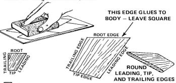
Fine-sand the balsa fin die-cut sheet (part G), then carefully remove the fins from the sheet. Free the edges with a sharp knife. Sand the leading, trailing, and fin tip edges round. Sand the root edge square.
