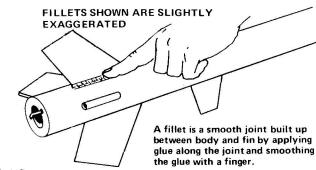
13 Reinforce the fin joints with glue. Holding the rocket horizontally (level), apply a line of glue to both sides of each joint. Smooth out the glue with your finger. Keep the rocket level until the glue dries.
