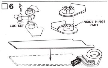
Remove the wing hinge halves from the plastic hinge/lug set (part G). Carefully sand the hinge part that goes inside the other half until the assembled parts rotate easily, but do not sand so much as to cause them to be too loose. Pull the two pieces apart and cement a wing hinge half to each wing with tube-type plastic cement, making sure the wing fits correctly into the area provided in the wing hinge half as shown. Allow these parts to dry thoroughly.
