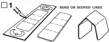
Carefully remove the parachute tube support from the die-cut card (part A). Use a modeling knife to free the part from the sheet. Bend it on the scored lines to the shape shown.
