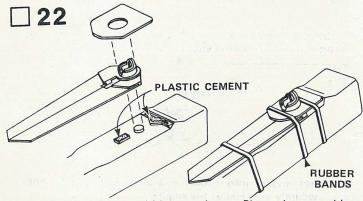
Assemble wing halves and hinge as shown. Place wing assembly on pivot point and place small amounts of tube-type plastic cement on the forward and rear retainer supports. Place plastic retainer plate in position. Make sure the cement doesn't get on hinge or hinge point. Wrap rubber bands around the body to hold the plate and wings in place until cement dries.
