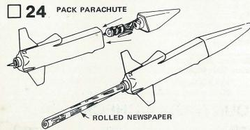
Push parachute and shock cord into parachute tube and slide nose cone into place. Roll up a piece of newspaper tight enough to go into the engine mount and slide it into the engine mount as shown. Using this as a paint handle apply two light coats of gloss white enamel spray paint. Allow each coat of paint to dry completely. Follow paint instructions on spray can for best results.
