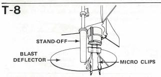
Slide launch rod through rocket launch lugs and place rocket on launch pad. Make sure the rocket slides freely on launch rod. Clean the micro-clips and attach them to the igniter wires. Arrange the clips so they do not touch each other or the metal blast deflector. Attach clips as close to engine as possible.
