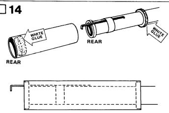
Apply a line of glue to the forward adapter ring and the inside of one reactor body tube (part K) as shown. Slide the reactor tube into place, matching its ends with the adapter rings. Wipe away any exposed glue.
