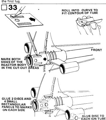
Cut out the shaded areas from the reactor detail template. Pre-form the template, and mark both sides of the reactor body in the cutout areas. Glue two discs and four small rectangular panels to the locations marked. Glue two more discs centered on the alignment line on the ion tubes near the rear edge of the tube. Glue the remaining two discs to the secondary tube top and bottom alignment lines near the front edge of the tube.
