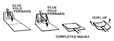
Cut out the shock cord mount (part N). Fold on dotted lines, then unfold and apply glue to Section 1. Lay the end of the shock cord (part M) in the glue. Fold over and apply glue to the back of Section 1 and the exposed portion of Section 2. Fold again to complete the mount. Curl the edges of the mount up so it will match the contour of the body tube and hold with your fingers until the glue sets.
