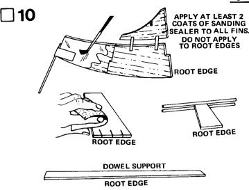
Apply a coat of sanding sealer to all surfaces of wood parts except root edges (edges that glue to tubes or dowels). Allow sealer to dry, then lightly sand parts. Repeat sealing and sanding steps a second time. Repeat until tiny grain lines in the wood are filled and everything looks and feels smooth.
