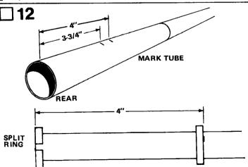
Mark the rear end of the body assembly 3-3/4" and 4" from the end. Apply a line of glue around the tube at the 3-3/4" mark and slide one of the adapter rings (part H) onto the tube until the front end of the ring is even with the 4" mark. Wipe away any excess glue immediately. Glue the split adapter ring (part I) to the tube so it is even with the rear end.
