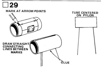
Cut out the ion tube marking guide from the pattern sheet. Wrap it around an ion tube (part O) and mark at each arrow point. Repeat with the other ion tube. Draw straight connecting lines between marks. Apply glue to end of the pylon and center the tube on the pylon and the alignment lines.
