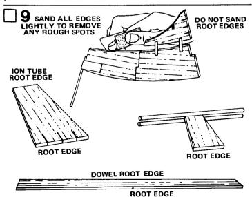
Fine-sand both sides of each wood part and all outside edges THAT ARE NOT ROOT EDGES to remove any rough spots and mismatch in glue joints.
