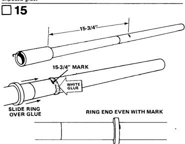
Mark the main body tube 15-3/4" from the front of the reactor body tube. Slide an adapter ring down the main body past the 15-3/4" mark. Apply a line of glue around the main body at the mark and slide the adapter ring up until the rear end of the ring is even with the mark.
