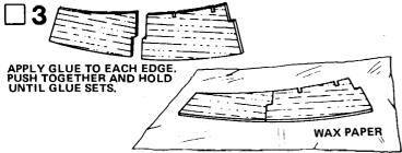
Glue the sails together as shown, making sure you match one notched and one unnotched half. Lay the sail assemblies flat on a piece of waxed paper and weight down to hold in position while the glue dries.
