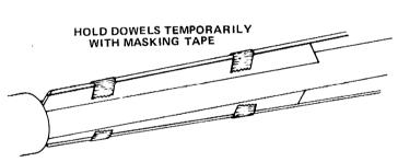
Test-fit the 1/8" diameter dowels used in Step 4 between the sails and the dowel supports. Trim the dowels to the correct length. For best results, cut the dowels 1/32" to 1/26" longer than needed and then match to the sail and supports by sanding the ends. Glue the dowels to the sails and supports. Temporarily tape each dowel in position with a short piece of masking tape until glue sets. DO NOT wait until the glue is completely dry or tape will stick.
