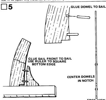
Glue dowel pieces to sail and then glue front sail part to dowels as shown. Make sure dowel pieces are centered in each of the notches. Set bottom edges of the parts against a ruler to make sure they are straight.
