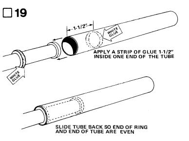
Smear a band of glue around the inside of the parachute compartment tube (part L), 1-1/2" inside one end of the tube. Apply glue around the outside of ring as shown. Slide end of the tube with glue inside, onto the rings until the end of the tube and end of the ring are even. Wipe away excess glue.
