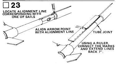
Cut out the main body tube marking guide from the pattern sheet and wrap it around the main body tube just behind the secondary tube. Locate the alignment line on the secondary tube that is in line with a sail and align one of the arrow points on the guide with this line as shown. Mark at each arrow point as shown. Use a ruler to draw a straight connecting line between each matching pair of marks. Extend the lines back from the rear of the secondary tube about 7".
