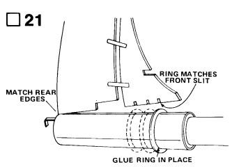
Position the front radiator ring (from the die-cut card) on the reactor body using a sail for a guide. The ring should match the front slit on the sail when the rear of the sail is even with the rear of the reactor body. Glue the ring to the body in this position. A drop or two of glue is sufficient — do not over-glue. Use the sail to make sure the ring is correctly positioned all around the body. Slip the other two rings onto the reactor body in their approximate positions, but do not glue.
