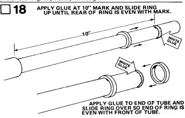
Mark the main body tube 10" from the front of the secondary tube. Slide another ring past the 10" mark. Apply a line of glue around body tube and slide the adapter ring up until the rear of the ring is even with the mark. Apply a line of glue around the front end of the main tube and slide the remaining adapter ring over glue, so front end of ring is even with front end of tube.
