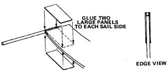
Mark the two remaining 2" dowels 3/4" from one end. Apply a line of glue along one edge of a dowel to the 3/4" mark and apply dowel to the top edge of each sail as shown. After glue sets, apply glue to the back sides of the large panels from the die-cut card and position them as shown on the sides of each sail.
