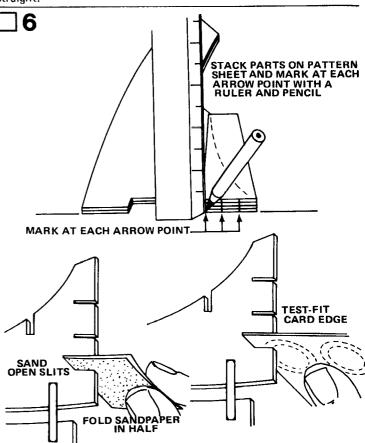
The sail fronts and engine pylons each have three slits die-cut in their root edges. Stack these four parts so the slits match. If the slits do not show up, stack the four parts on the illustration on the pattern sheet (part C) and mark the root edges at the arrow points as shown. Fold a piece of extra-fine sandpaper and use it to open the slits until the die-cut card material (part D) fits snugly in the slits.
