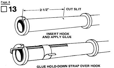
Cut a 1/8" slit in the body, directly in line with the gap in the split adapter ring, 2-1/2" from the end of the body. Cut out the hold-down strap from the pattern sheet. Insert one end of the engine hook (part J) into the slit and lay the hook along the body so the other end passes through the gap in the split ring. Smear glue over one side of the hold-down strap and wrap it around the body, centered over the hook. Apply a drop of glue over the forward end of the engine hook.
