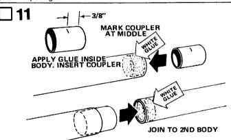
Assemble the main body. Mark the tube coupler (part F) at its middle. Smear glue around the inside of one end of an 18" body tube (part G). Insert the coupler into the glued body end so half of the coupler is in the tube. Let the glue set, then smear glue inside one end of the other 18" tube and slide glued end onto the coupler to join the tubes. Lay the assembly on a flat table top and roll gently to make sure the tubes are straight.
