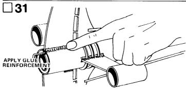
When all the glue joints have dried, apply a glue reinforcement to each sail, pylon, support, and body tube joint. Holding the model horizontally, apply a line of glue to the joint and smooth it out with your finger. Support the rocket horizontally while the glue dries.
