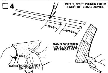
Cut two 9/16" long pieces from each of the two 18" long 1/8" wood dowels (part B). Sand round each end of the four dowel pieces. After the glue has dried on the sail, test-fit the 9/16" long
