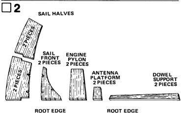
Sort and identify the parts as shown. Make sure all mating edges match on the sail halves.
