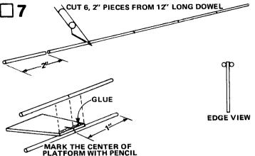
Cut the 12" long dowel (part E) into six 2" pieces. Glue two pieces to the end of each antenna platform. The 2" dowel antennas should be perfectly centered on the ends of the platforms as shown.
