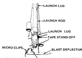
Slide the launch lugs of rocket onto the launch rod. Make sure rocket slides freely on the launch rod. If the launch pad you are using does not have a rocket stand-off, place a piece of masking tape on rod as shown to keep rocket 1" above the deflector plate. Clean micro-clips, attach them to the igniter wires as close to engine nozzle as possible. Arrange the clips so they do not touch each other or the metal blast deflector.
