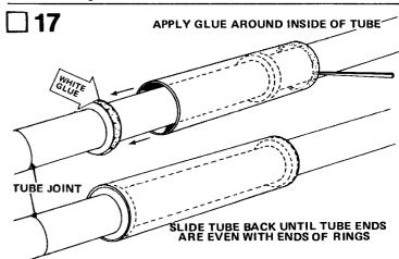
Slide the 4" long secondary body tube onto the forward ring and almost to the next adapter ring. Use a toothpick or short dowel scrap to apply a ring of glue just inside the front end of the tube. Apply glue around the outside of the second ring, then slide the tube back over the ring until the end of the tube is even with the end of the ring. Wipe away excess glue.
