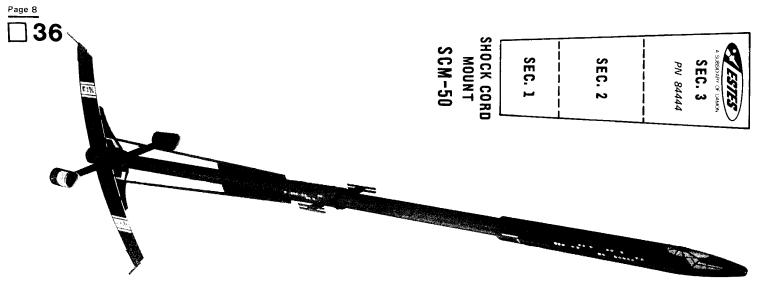
Apply decals (part U) in positions shown in the photograph above and on the color panel. To apply decals cut only one decal at a time from the sheet. Submerge decal in water for 15 to 20 seconds (until decal slides on backing sheet). Gently slide decal from backing sheet and onto the model. Move decal into exact position and carefully blot away excess water with a soft cloth. If the decal "sticks"
