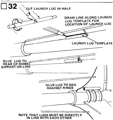
Cut out the launch lug location template from the pattern sheet. Mark the lug location on the dowel support as shown. Cut the
