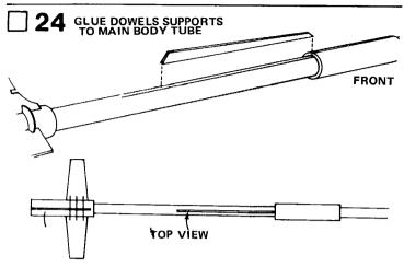
Glue the dowel supports to the main body on the lines drawn in Step 23, with the small end of the supports directly behind the secondary tube. Sight along the model from the front and adjust the supports so they are aligned with the sails.
