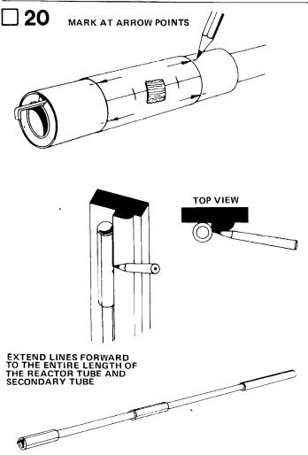
Cut out the reactor body tube marking guide from the pattern sheet. Wrap it around the reactor body and mark at each arrow point as shown. Draw straight lines connecting each mark. A door frame inside edge can be used as a guide. Extend the lines the full length of the reactor tube, and without moving the tube, draw corresponding lines the full length of the secondary tube.
