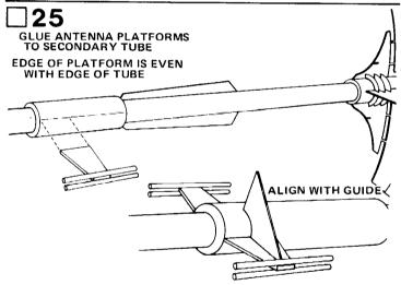
Glue the antenna platforms to the secondary body tube. The front edge of each platform should be even with the front edge of the secondary tube as shown. Use the alignment guide used in Step 22 to be sure the antenna platforms project straight out from the tube.
