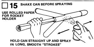
Insert a sheet of rolled up newspaper into the rear of the rocket as shown. Apply two or three coats of gloss orange spray paint to the entire model. Allow each coat to dry thoroughly before applying the next coat.
