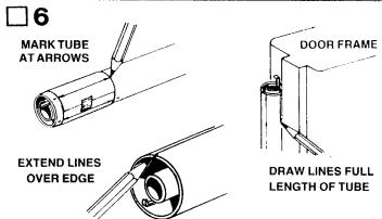
Cut out the tube marking guide from the pattern sheet (part F) and wrap it around the body tube. Line up the engine hook with the launch lug alignment line on the marking guide. Mark the body tube at each of the arrow points. Draw straight lines connecting each pair of marks. A door frame inside edge can be used as a guide as shown. Extend the lines down full length of tube. Extend the lines over the edge of the tube as shown.
