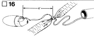
Using a double knot, tie the shock cord around the middle of the plastic streamer (part L) about 2" from the end of the shock cord. Attach the free end of the shock cord to the nose cone with a firm knot.
