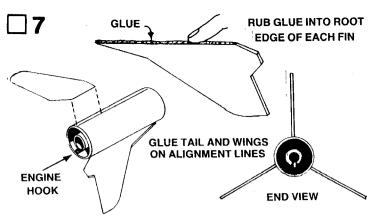
Rub glue into the root edge of each wing and the tail and allow to dry. Apply glue to the wings and tail again and position wings and tail on the alignment lines in positions shown. Adjust the wings and tail so they project straight away from the body tube. DO NOT set the rocket on its wings and tail while the glue is wet.
