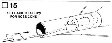
Apply glue to the side of the shock cord mount and press the mount firmly into position as far as possible down inside the body tube. This will allow clearance for the nose cone to fit into place. To insure a good bond use a stick or your finger to smear a film of glue over the shock cord mount and surrounding area in the body tube.
