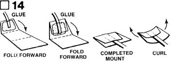
Cut out the shock cord mount from the parts illustration on front of instructions. Fold on dotted lines, then unfold and apply glue to Section 1. Lay the end of the shock cord (part K) into the glue. Fold over and apply glue to the back of Section 1 and the exposed portion of Section 2. Fold again to complete mount. Curl the edges of the mount up so it will match the contour of the body tube and hold with your fingers until the glue sets.
