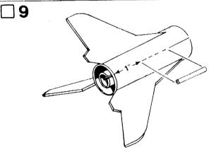
Glue launch lug (part I) to rocket body tube on the launch lug line. The rear of the launch lug should be 1" from the rear of the rocket body tube. Align the launch lug straight along the body
