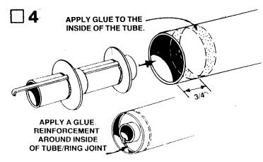
Test-fit engine mount into the body tube (part E) as shown. Sand if necessary to assure a smooth fit. Remove and apply a ring of glue around the inside of the rear of the body tube. Replace engine mount quickly, before glue sets, so that the rear of the engine mount tube is even with the end of the body tube. Apply a glue reinforcement to tube/ring joint.
