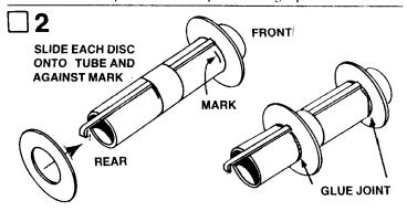
Remove the centering rings from die-cut ring set. (part C). Slide one ring onto the engine mount tube from the front until it is even with the 2-1/4" mark. Slide the remaining centering ring onto the rear of engine mount tube until it is even with the 1" mark. Apply a line of glue at the ring/tube joints on both sides of each ring. Set aside until glue is completely dry.
