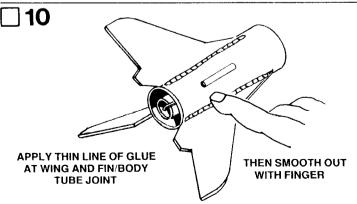
When the glue on the fin joints has dried, apply a glue reinforcement to each wing and tail body tube joint. Holding the model level, apply a line of glue to both sides of each wing and tail joint and on both sides of the launch lug. Smooth out the glue with your finger. Support rocket level (Do not stand it on the fins) until the glue dries.
