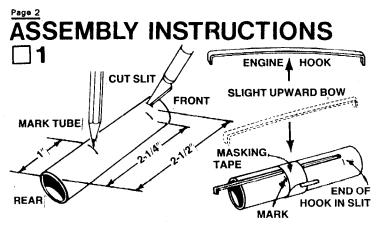
Mark the engine mount tube (part A) 1", 2-1/4", and 2-1/2" from one end. Cut a 1/8" long slit at the 2-1/2" mark. Gently bend the engine hook (part B) so it bows upward very slightly in the middle. (Don't bend the wrong way.) Insert one end of the engine hook into the slit in the tube. Hold hook in place with a wrap of masking tape.
