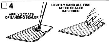
Apply a coat of sanding sealer to each fin. Apply sealer to all edges except the root edge. When sealer is dry, lightly sand all the sealed surfaces. Repeat sealing and sanding process until balsa grain no longer shows. Resand root edge, lightly, to remove any trace of sealer.
