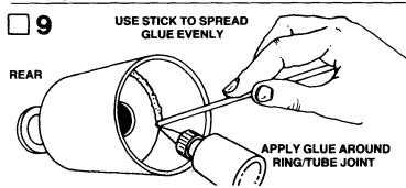
Apply a line of white glue around the forward centering ring where it meets the body tube. Stand the tube upright while glue dries. Check to be sure that there are no gaps or holes in the glue joint when dry. Apply more glue if necessary.
