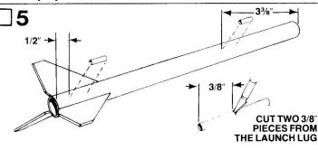
Cut two (2) 3/8" pieces from the launch lug (part H) with a modeling knife or single edge razor blade. Make marks on the lower (large) body tube launch lug line at 1/2" from the rear, and 3%" from the front. Glue the launch lugs in place as shown in the illustration.
