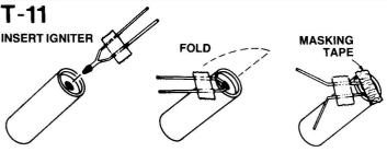
Select an engine and install an igniter as directed in the engine instructions. Use an A8-5 for first flight.
