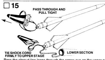
Pass the shroud line loops through the screw eye on the upper section. Pass the parachute through the loop ends and pull the lines tight against the screw eye. Tie the free end of the shock cord firmly to the screw eye. A square knot or strong double knot should be used.
