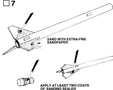
When all the glue on the model is dry, prepare the balsa parts for painting. Apply at least two coats of sanding sealer to all balsa surfaces. Let dry and sand thoroughly with the extra-fine grit sandpaper after each coat. Do this until all the tiny grain lines in the wood are filled and ev-
