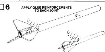
When the glue on the fin joints and launch lugs has dried, apply a glue reinforcement to each joint. Holding the model level, apply a narrow line of glue to both sides of each fin joint and the launch lugs. Smooth out the glue with your finger. Be sure there is no excess glue in front of or behind the launch lugs. Keep the sections level until the glue dries.
