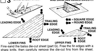
Stack fins together as shown and sand all four sides as illustrated. Lightly sand both sides of each fin. Sand the leading edge and trailing edge of each fin to make them round. Leave the root (body) edge sanded "flat". The root edge may be identified by careful comparison with the drawings. Sand large fins first, then sand the small fins separately.
