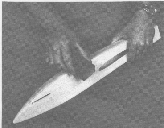
Complete the top and bottom sheeting and sand the corners to shape
