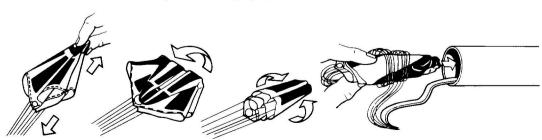
3. Install the nose cone into the forward end of the rocket body. Be certain the fit is neither too loose or too tight. If the nose cone falls out of the rocket body when the model is pointed downward, the fit is too loose. If while pointed downward, the nose cone can't be shaken out of the tube, the fit is too tight. If too loose, wrap tape around shoulder for snug fit. If too tight, lightly sand shoulder slightly for looser fit.
