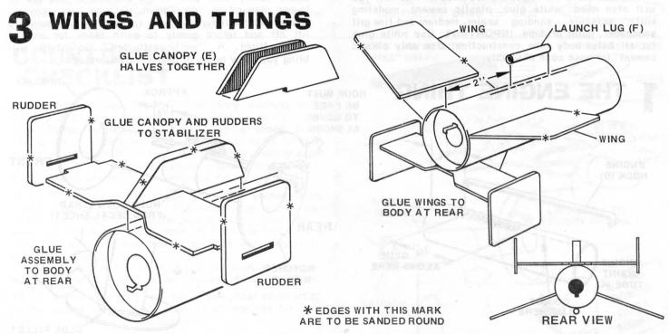
Glue the two canopy pieces together. Sand round all balsa edges as noted by this mark (\*) in drawing. (You may wish to sand part sides smooth before removing them from balsa sheets.) Glue the canopy to the stabilizer on its centering lines.
