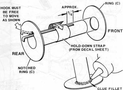
Tightly wrap the hold-down strap (from decal sheet) around the hook and tube as shown. Center the notched paper ring over the hook and glue to the tube REAR. Hook must be free to move as shown. Glue the other ring to the front of the tube. Run lines of glue (known as "glue fillets") around the front and rear ring/tube joints. Allow mount assembly to dry completely.
