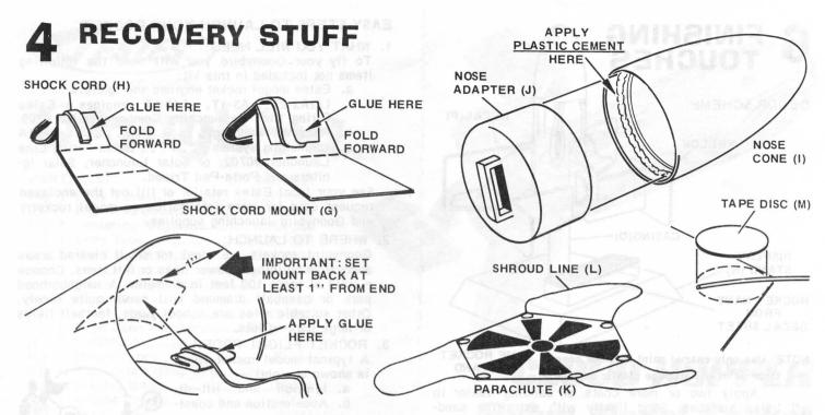
Cut out the shock cord mount and prefold along dotted lines. Apply glue to section 1 and lay shock cord end into glue. Fold this first section over. Spread glue over back of first section and exposed part of section 2. Lay shock cord as shown and fold over again. Clamp the unit together with your fingers until the glue sets. Apply glue to the mount as illustrated. Press the mount into position against the tube wall and hold it until the glue sets.
