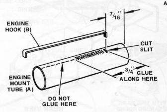
Cut a 1/8" slit in the engine mount tube, 7/16" from one end. Apply a drop of white glue to the slit and also straight along the tube for approximately 3/4". Push one end of the metal engine hook into the slit. Press the hook into the glue and align straight along the tube. Wipe away any excess glue.
