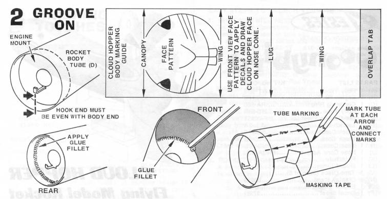
Insert engine mount into the rocket body tube. End of metal engine hook MUST be even with body tube end. (For quickest alignment, simply press body tube end against table top and engine mount will automatically move forward to align with tube end.)
