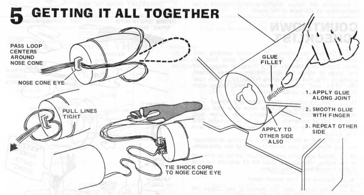
Pass the shroud line loop "centers" through the nose cone "eye". Now pass the loop centers around the nose cone as shown and pull lines tight to secure parachute. Tie the shock cord to the nose cone "eye".
