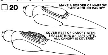
Mask off the canopy with masking tape, as shown, to protect it while spray painting the model.
