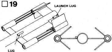
Glue the launch lugs (part P) to the body tube/fin joints as shown. Sight through the launch lugs to see that they are straight. If a launch rod is available, carefully slide the rod through the launch lugs to be sure that they are in line with each other.
