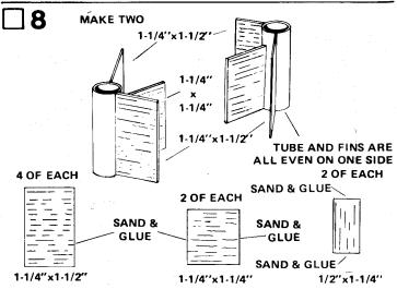
Separate the fins into the three sizes. Sand the edges of each which will be glued, to remove the sanding sealer on those edges. Rub a line of glue into the edges of each fin as illustrated. NOTE: Pay close attention to the direction of the grain on each of the fins. Allow the glue to dry. Glue one of the 1-1/4" x 1-1/4" fins to the middle line of the larger 1-1/2" long body tubes so that the rear of
