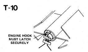
Insert engine into rocket engine mount. Engine hook must latch securely over end of the engine.
