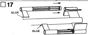
Rub a line of glue onto the root edges of the fins on the dowel units. Slide (do not glue) the rear of the dowel units into the rear fin units until the ring and tube end are even. Adjust the units until the front and rear fins are in line with each other. Press the fins onto the alignment lines and hold in place until the glue sets. Stand the rocket on end and allow the glue to dry completely before proceeding.
