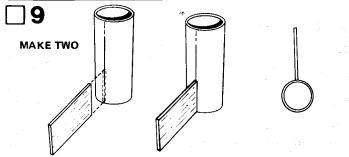
Glue one of the 1-1/4" x 1/2" fins to one of the large 1-1/2" long body tubes, on one of the alignment lines, so that the rear of the fin and the rear of the body tube are even as shown. Adjust the fin so that it projects straight away from the tube. Stand the tube on end to dry. Repeat this process for the remaining large body tube and small fin.
