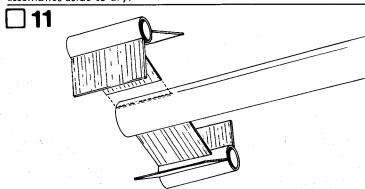
Glue the rear fin assemblies to the main body tube as shown. Make sure the fins are properly positioned on the alignment lines and the rear of the fins are even with the rear of the body tube. Stand the rocket up on a flat surface and adjust the fins so that they project straight away from the body tube. A piece of wax paper may be used under the rocket to prevent gluing it to the surface. Allow the unit to dry completely.
