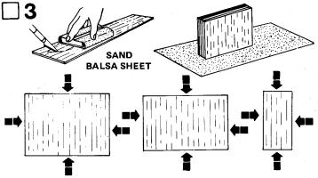
Fine-sand the balsa die-cut sheet (part D). Free the fin edges with a sharp knife, then carefully remove the fin die-cuts from the sheet. Stack the fins into three sets as shown. Sand all of the fin edges square as shown. Lightly sand both sides of each fin. Leave all of the fin edges square.
