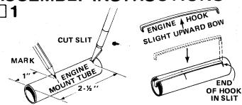
Mark the engine mount tube (part A) at 1" and 2-1/2" from one end. Cut a 1/8" long slit at the 2-1/2" mark. Gently bend the engine hook (part B) so that it bows upward very slightly in the middle. (Study the drawing — Don't bend the wrong way.) Insert one end of the engine hook into the slit in the tube.
