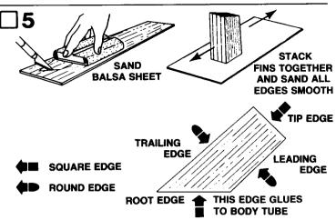
Fine-sand the balsa die-cut sheet (part F). Free the fin edges with a sharp knife, then carefully remove the die-cut fins from the sheet. Stack fins together as shown and sand all four sides as illustrated. Lightly sand both sides of each fin. Sand the leading edge and trailing edge of each fin to make them round. Leave the root (body) edge and tip edge square. The root edge may be identified by careful comparison with the drawings.
