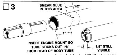
Test-fit the engine mount into the body tube (part D). Sand adapter ring if necessary to assure a smooth fit. Apply a ring of glue around the inside of the rear of the body tube about 1" from the end of the tube. Make certain that the engine hook is to the rear and insert the engine mount with one smooth motion. Do not pause, or the glue may "lock" with the engine mount in wrong position.
