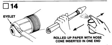
Trim away the excess plastic from nose cone eyelet and from around the nose cone (part J). Spray paint the nose cone with several light coats of blue spray enamel paint. The nose cone can be supported by wrapping newspaper around the shoulder of the nose cone and securing it with masking tape.
