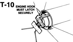
Insert engine into rocket engine mount. Engine hook must latch securely over end of the engine.
