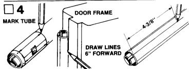
Cut out the body tube marking guide from the pattern sheet (part E) and wrap it around the body tube. Place the marking guide so that the engine hook lines up with the arrow points labeled launch lug. Mark the body tube at each of the arrow points. Draw straight lines connecting each pair of marks. A door frame inside edge can be used as a
