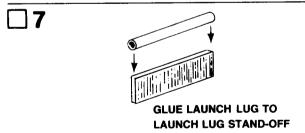
Locate launch lug stand-off on balsa die-cut sheet. Sand all edges square. Apply glue to one edge of launch lug stand-off and position the launch lug (part B) on it. Make sure launch lug is straight with the stand-off.
