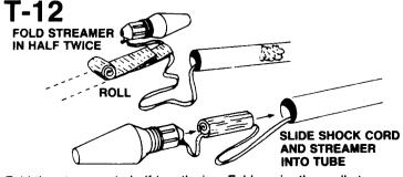
Fold the streamer in half lengthwise. Fold again, then roll streamer tightly until the streamer fits loosely into the rocket body. Pack the shock cord neatly into the rocket body. Slide nose cone into place.
