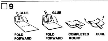
Cut out the shock cord mount (part H). Fold on dotted lines, then unfold and apply glue to Section 1. Lay the end of the shock cord (part I) into the glue. Fold over and apply glue to the back of Section 1 and the exposed portion of Section 2. Fold again to complete mount. Curl the edges of the mount up so it will match the contour of the body tube and hold with your fingers until the glue sets.
