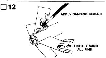
Proper application of sanding sealer makes the rocket look better and reduces drag so that the rocket will fly higher. However, this step is not essential to make a safe, attractive rocket. Apply a coat of sanding sealer to each fin. When sealer is dry, lightly sand all the sealed surfaces. Repeat sealing and sanding process until balsa grain is filled and smooth.
