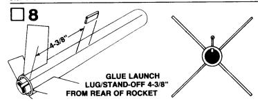
Glue launch lug/stand-off to rocket body tube on the launch lug line. The rear of the stand-off should be 4-3/8" from the rear of the rocket.
