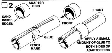
Sand the inside edges of the adapter ring (part C) to remove burrs. The ring should slide easily onto the engine mount tube. Slip the ring onto the front end of the engine mount tube and slide it down to the 1" mark. Make sure the engine hook runs straight down the tube. Then apply glue to both sides of the adapter ring.
