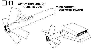
When the glue on the fin joints has dried, apply a glue reinforcement to each fin/body tube joint. Holding the model level, apply a line of glue to both sides of each fin joint and on both sides of the launch lug/stand-off. Smooth out the glue with your finger. IMPORTANT: Support rocket on table edge as shown until the glue dries.
