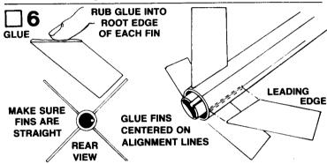
Rub glue into the root edge of each fin and allow to dry. Apply glue to the fins again and position fins on the alignment lines in positions shown. Adjust the fins so they project straight away from the body tube. DO NOT set the rocket on its fins while the glue is wet.
