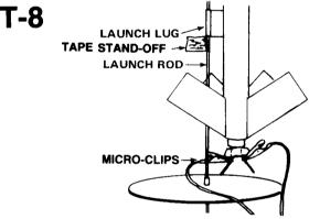
Slide launch rod through rocket launch lug and place rocket on launch pad. Make sure the rocket slides freely on the launch rod. Clean the micro-clips and attach them to the igniter wires. Arrange the clips so they do not touch each other or the metal blast deflector. Attach clips as close to protective tape on igniter as possible.
