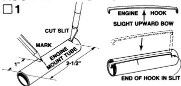
Mark the engine mount tube (part A) at 1" and 2-1/2" from one end. Cut a 1/8" long slit at the 2-1/2" mark. Gently bend the engine hook (part B) so that it bows upward very slightly in the middle. (Study the drawing—Don't bend the wrong way.) Insert one end of the engine hook into the slit in the tube.
