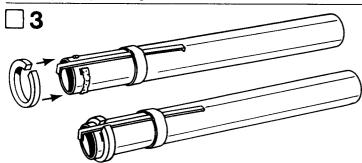
Apply a bead of glue around the rear of the tube just forward of the 1/8" mark. Do not get glue on the engine hook. Slide the split adapter ring (part D) over the rear of the tube and push forward until the rear of the ring is even with the mark. Make sure the engine hook is centered in the split portion of the ring. Hold the ring in place until the glue sets.
