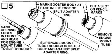
Wrap a piece of sandpaper around a wood dowel or pencil and sand out the openings at the front and rear of the booster body until the engine mount tube slips through booster body. Slide engine mount tube through booster body and up against split adapter ring. Hold the two parts together and mark, along inside edges of split adapter ring, on booster body with a pencil. Remove engine mount tube and cut, on the marks, a slot in the plastic edge of the booster body.
