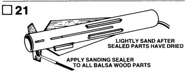
Apply a coat of sanding sealer to all balsa wood parts. When sealer is dry, lightly sand all the sealed surfaces. Repeat sealing and sanding process until balsa grain is filled and smooth.
