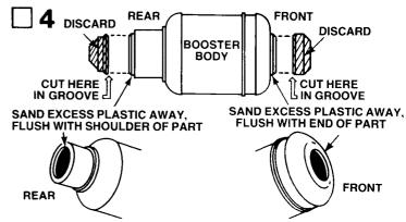
Cut the ends from the molded booster body (part E) as shown and discard. Use a modeling razor saw, or a fine woods coping saw to cut through the separation grooves as shown. Make repeated light cuts around the groove work slowly to avoid tearing or marring the plastic part. Using an emery board or sanding block, sand excess plastic lip away at the front and rear of the part.
