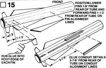
Rub glue into the root edge of each fin as stated in step 6 and position as shown on alignment lines noted with the letter "F", lower fins 1/8" from the rear of tube, forward fins 1-1/2" from rear of tube. Adjust fins so they project straight away from body tube and are 90° to one another. Glue conduit details 3-7/8" from rear of tube on the conduit alignment lines. DO NOT set the upper stage body on its fins while glue is wet.
