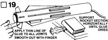
When the glue joints have dried, apply a glue reinforcement to each fin body tube joint, around launch lug, and around each conduit detail. Holding the model level, apply a line of glue to the joint, then smooth out the glue with your finger and wipe away any excess glue. <a href="MPORTANT">IMPORTANT</a> — Support rocket section level, or horizontally, on table edge until glue dries.
