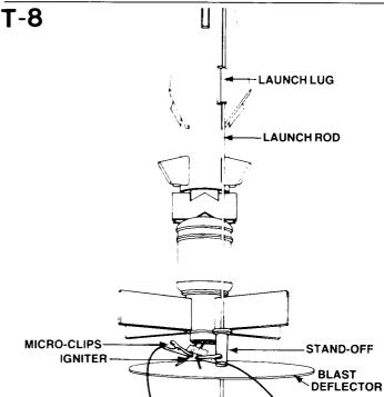
Slide the launch rod through rocket launch lug and place rocket on launch pad. Make sure the rocket slides freely on the launch rod. Clean the micro-clips and attach them to the igniter wires. Arrange the clips so they do not touch each other or the metal blast deflector. Attach clips as close to protective tape on igniter as possible.
