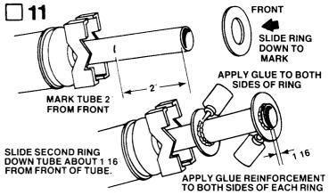
Mark the booster tube 2" from the front of the tube. Remove the centering rings from the ring set (part H). Slide one ring down to the mark and apply a bead of glue to both sides of ring joint. Slide second ring down front of tube about 1/16" from edge of tube. Apply glue to both sides of ring joint.
