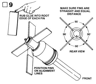
Rub glue into the root edge of each fin and allow to dry. Apply glue to the fins again and position fins on the alignmnet lines in positions shown. Adjust the fins so they project straight away from body tube and are 90° to one another. DO NOT set the rocket booster on its fins while glue is wet.
