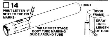
Cut out the upper stage body tube marking guide from the pattern sheet. Wrap it around the upper stage body tube (part I) and secure it with masking tape. Mark the body tube at each arrow point. Print the letter "F" next to each of the four rear fin marks. Remove the marking guide and draw straight lines connecting each pair of marks. Extend the lines the length of the tube.
