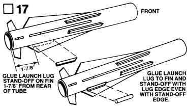
Locate launch lug stand-off, and rub glue into edge and side. Apply glue to edge and side again and position 1-7/8" from rear edge of tube, as shown, on one of the fins. Apply glue to launch lug (part K) and position on fin and stand-off with lug edge even with stand-off edge.
