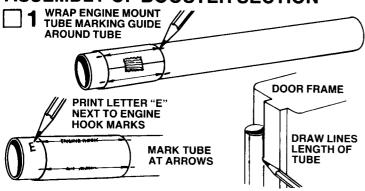
Cut out engine tube marking guide from the pattern sheet on separate instruction sheet and wrap it around the engine tube (part A) and secure it with masking tape. Mark the engine tube at each of the arrow points. Print the letter "E" next to the engine hook marks to identify engine hook location. Remove the marking guide and draw straight lines connecting each pair of marks. A door frame inside edge can be used as a guide as shown. Extend the lines the length of the tube.
