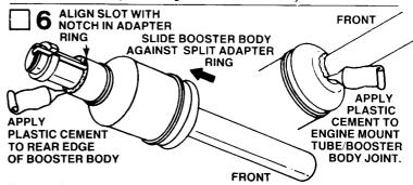
Apply a bead of plastic cement to the rear edge of the booster body. Push booster body down engine mount tube and against split adapter ring. Carefully align slot in edge of booster body with notch in split adapter ring. Wipe off excess cement from joint and hold in place until cement sets. Apply a bead of cement to front of booster body/engine mount joint as a reinforcement, and wipe away excess cement with your finger.
