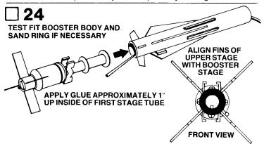
When paint is dry on both sections of rocket, remove parachute and nose cone from upper stage, test fit booster section into upper stage body. Sand rings if necessary to assure a smooth fit. Remove booster section, apply glue around the inside surface of upper stage body tube
