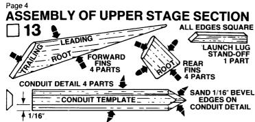
Remove the remaining die-cut balsa parts from the die-cut sheet. Stack like parts together and sand edges smooth then separate, and sand leading edge and trailing edges of each forward fin, and rear fin round. Sand all edges square and smooth on launch lug stand-off. Refer to the full scale conduit template above to sand a 1/16" beveled edge on all four conduit details.
