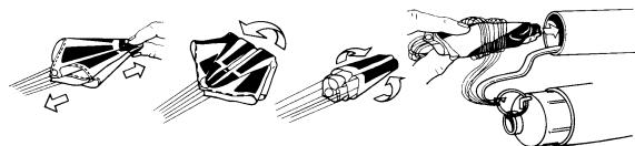
3. Install the nose cone into the forward end of the rocket body. Be certain the fit is neither too loose or too tight. If the nose cone falls out of the rocket body when the model is pointed downward, the fit is too loose. If, while pointed downward, the nose cone can't be shaken out of the tube, the fit is too tight. If too loose, wrap tape around shoulder for snug fit. If too tight, lightly sand the shoulder slightly for looser fit.
