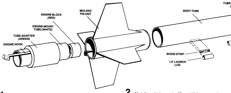
Mark the engine mount tube 25 mm (1") from one end. Cut a 3 mm (1/8") wide slot at the mark. Apply glue inside this end of the tube and insert the red engine block until even with the tube end. Insert the engine hook in the slot. Apply glue around the outside of the engine mount tube. Slide the green adapter ring onto the tube and over the glue, centering it on the engine mount tube.
