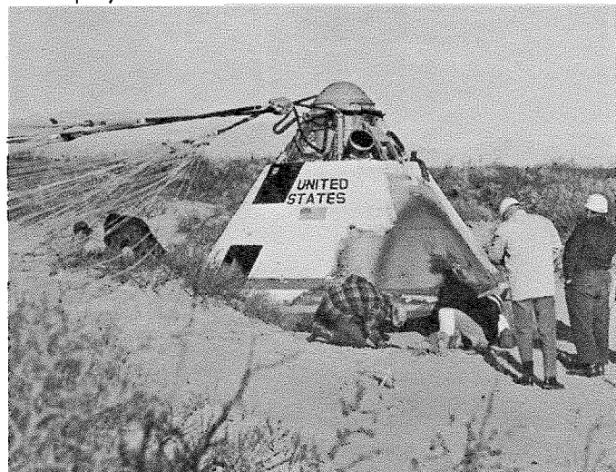
ENGINEERING INSPECTION AFTER DOWN-RANGE RECOVERY (NASA Photo S-64-35843)
