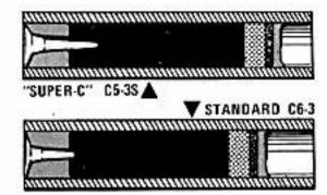
ENGINE CONSTRUCTION: The "SUPER-C" engines IC5 series) are modifications of the popular standard C6 series. The cutaway drawings above illustrate the major differences of "SUPER-C": larger nozzle opening, nozzle cored deeper into the propellant grain and slightly more fuel. The "SUPER-C" is in the same size casing as standard engines. They fit regular engine mounts and require
