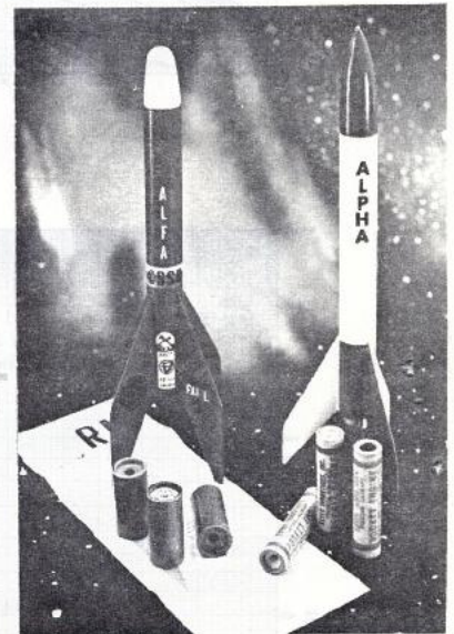
Czechoslovakian ALFA compares in size with the Estes ALPHA kit. Their engines, larger in diameter but shorter than ours, provide the same power as a B engine.
