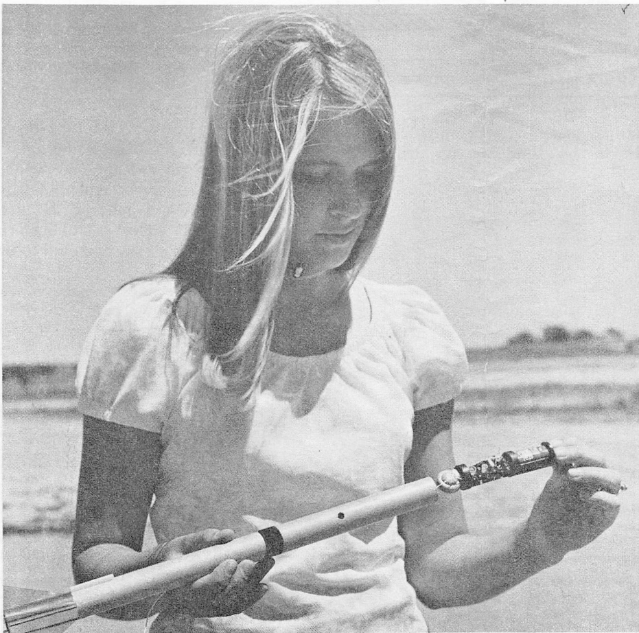
Jo Angel, a member of the Estes Rocketeer Communications Department staff, is shown placing a TRANSROC (in the microphone mode) in the payload compartment of a rocket. Hole in payload section is for tuning antenna-matching coil.
