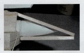
Once the fit is checked, then apply a line of glue across the front edge of the Nose
