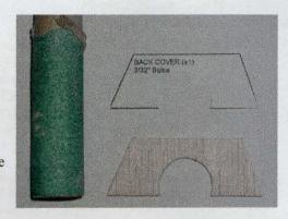
Test fit the template to the back of the rocket. Using the template cut out the Back Cover from the 2mm (3/32") balsa wood. Use sandpaper on a dowel to get the proper fit around the 18mm hole.
