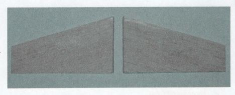
Optional: You may want to strengthen the Lower Wings by covering both sides Tracing Paper. Or you may choose just to soak the Lower Wing in CA. There are many tips on EMRR about strengthening fins, BUT, two important points. Do it in the LIGHTEST way possible (don't glass it) and also using Wax Paper and weight to keep this fin from warping. **NOTE:** The picture shows the use Tracing Paper.
