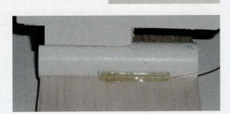
Once dry, stuff the Kevlar into the motor tube to keep it out of the way for future assembly.
