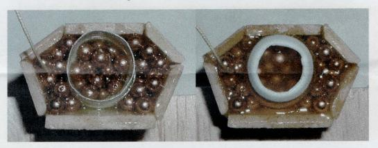
Add additional BB's until they are "packed" to be even with the balsa ends. The BB's in the plastic nose cone should also only be level with the balsa. Do not fill up in the plastic shoulder. They should not be sticking up over the edges. Mix up some epoxy and "drip" it into the nose cone from the end of a tooth pick over the BB's. The objective is to get enough epoxy in to fill the spaces between the BB's.
