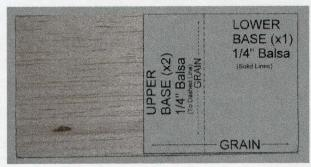
Cut out the Lower Base Template. DO NOT cut along the dashed lines for the Upper Base. Position the Lower Base Template on the 1/4" balsa wood so that the grain line matches the grain of the wood. Ensure the one edge is even with the edge of the balsa. The upper and lower edges should be equal with the sides of the balsa piece. Mark the balsa for the cut. Use the T-Square to cut a straight line. Be sure to take multiple passes cutting through just a little at a time.
