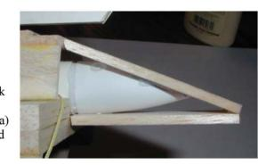
Once the fit is checked, then apply a line of glue across the front edge of the Nose Cone Bottom (balsa) where it will meet the Nose Cone Top (balsa). Then run a line of CA in the center of the Nose Cone Bottom (balsa) where it will touch the plastic Nose Cone. Then place in position and hold until tacked.
