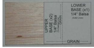
Cut out the Lower Base Template. DO NOT cut along the dashed lines for the Upper Base. Position the Lower Base Template on the ½" balsa wood so that the grain line matches the grain of the wood. Ensure the one edge is even with the edge of the balsa. The upper and lower edges should be equal with the sides of the balsa piece. Mark the balsa for the cut. Use the T-Square to cut a straight line. Be sure to take multiple passes cutting through just a little at a time.
