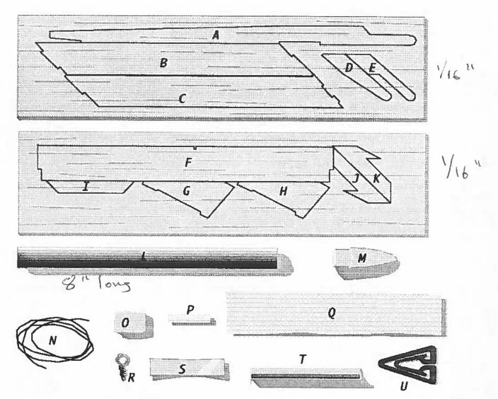
These are the parts for your model. The two balsa wood sheets have been die cut for you by Rol Klingberg at Future Flight out in California, so all the parts are already the right shape. Balsa parts A through H make up the glider. Balsa pieces I, J and K become parts of the pod.
