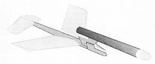
Now you have a completed airframe, and the first thing you should do is check the fit of the glider in the hook. The glider should slide right out when you hold the pod facing straight down. If it doesn't, sand a little between the tabs on the pod. After what you've been through, a little more sanding won't hurt you, but what's coming up just might. It is time to trim.
