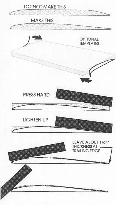
The most important thing is to have a smooth, gentle taper of the upper surface down to the trailing edge. It must not be a sudden, abrupt taper over the last half inch. If you get this part right, there isn't too much else you can do to mess up the wing. Even if you left the leading edge blunt, it might glide reasonably well.
