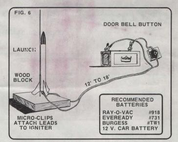
**CLUSTER IGNITION:** When igniting more than one engine at a time the igniters should be connected in parallel. To insure simultaneous ignition the power supply must be able to provide at least 6 amperes current at 12 volts <u>for each igniter</u> used. Generally a car battery in good condition is the best power supply. For further information on cluster ignition and building techniques see Estes Industries Technical Report TR-6.
