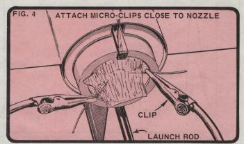
Slip the model's launch lug over the launch rod and lower the rocket into position on the launcher. Make sure the micro-clips on the launcher are clean, then clip one to each lead of the igniter. The clips must not touch each other and the igniter leads must not cross. If necessary, the rocket may be supported with a scrap of wood or an empty engine casing to make it easier to attach the clips and to keep the clips from touching the metal blast deflector and short circuiting.
