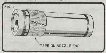
Always be sure the engine is mounted securely so its thrust will not move it forward in the rocket body. Extra care must be taken when mounting a Series II engine in the model. The engine block or engine holder must be securely glued in place. Be sure a force of ten pounds will not move the engine forward in the body. The engine should be positioned so its nozzle end is no more than 3/8'' forward from the end of the body tube.
